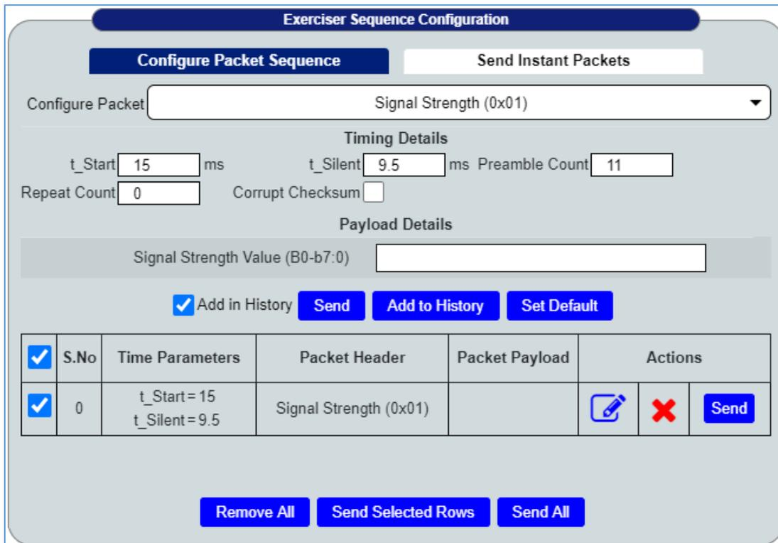
FIGURE 8.25: CONFIGURE AND SEND INSTANT PACKETS
