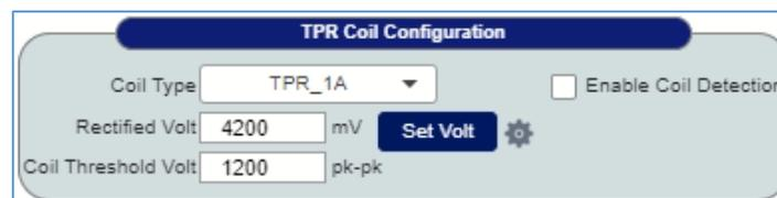
FIGURE 8.13: CONFIGURE TPR COIL
