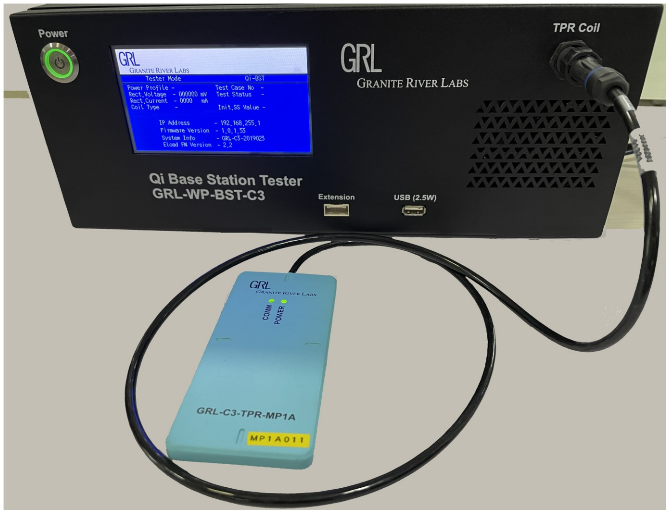
FIGURE 6.10: TPR COIL TO GRL-C3 CONNECTION
