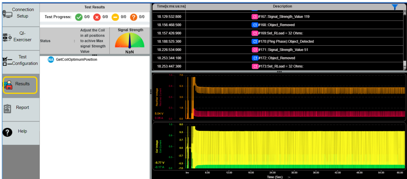
FIGURE 8.36: OPTIMUM COIL POSITION TEST EXECUTION EXAMPLE
