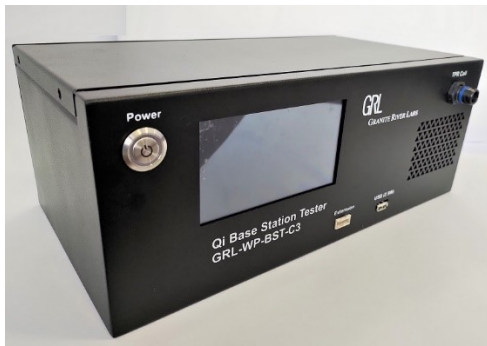
GRL-WP-BST-C3 – WPC Qi Wireless Charging Base Station Tester
