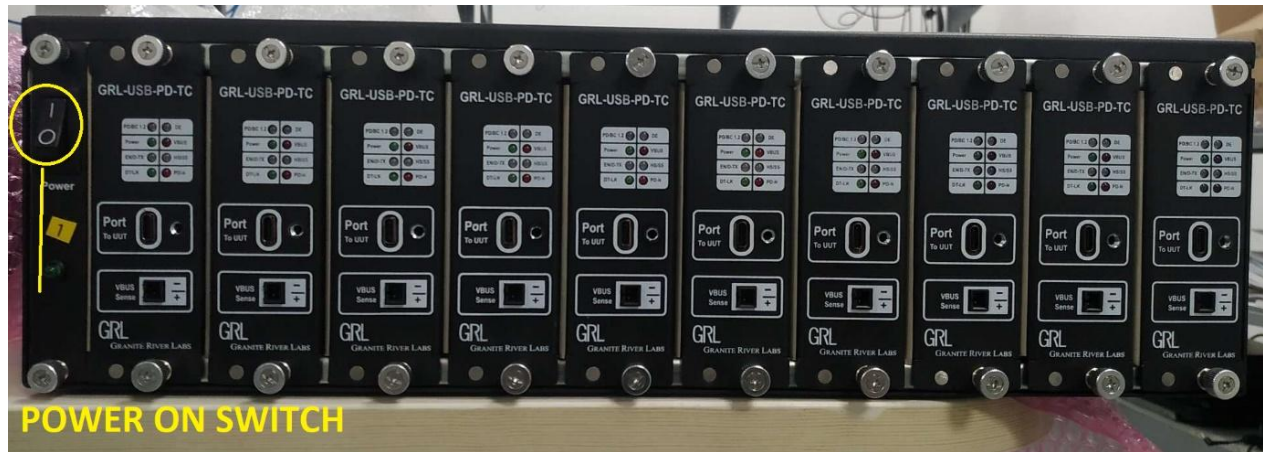
FIGURE 4.2: POWER ON GRL-V-UP TESTER
