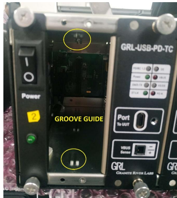
FIGURE 3.3: INSERT GRL TESTER CARD INTO TESTER
