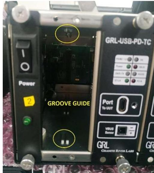
Figure 3. Insert GRL Tester Card Into Tester
