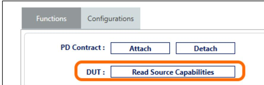
Figure 27. API Tab Functions Read Source Capabilities of DUT
