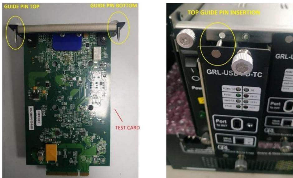
Figure 2. Check Orientation of GRL Tester Card Before Insertion
