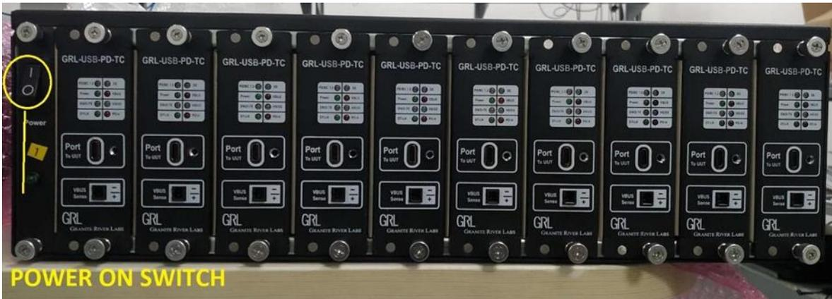
Figure 5. Power On GRL-V-UP Tester
