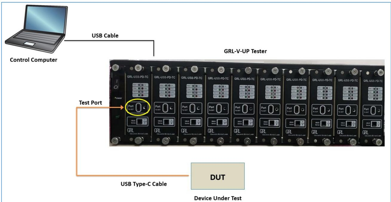
FIGURE 2.1: HARDWARE CONNECTION SETUP FOR GRL-V-UP API TEST SOFTWARE AND DEVICE UNDER TEST
