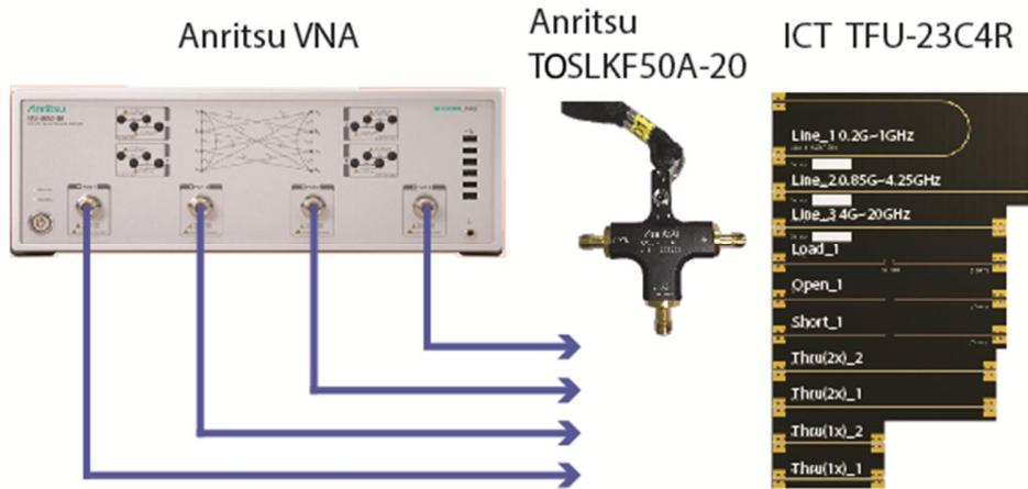
FIGURE 10. CALIBRATION SETUP FOR SOLT & DE-EMBEDDING CALIBRATION METHOD
