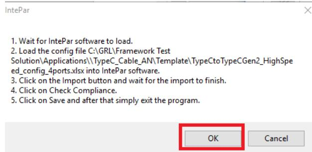
FIGURE 26. RUN AND COMPLETE INTEPAR TEST ANALYSIS
