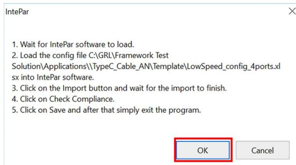
FIGURE 31. RUN AND COMPLETE INTEPAR TEST ANALYSIS
