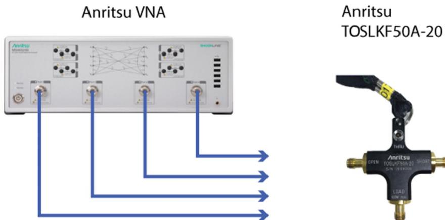
FIGURE 8. CALIBRATION SETUP FOR SOLT CALIBRATION METHOD
