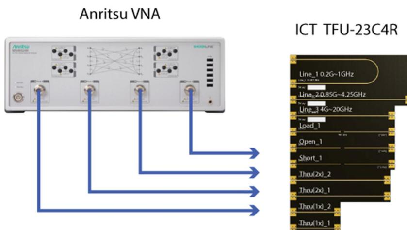
FIGURE 11. CALIBRATION SETUP FOR TRL CALIBRATION METHOD
