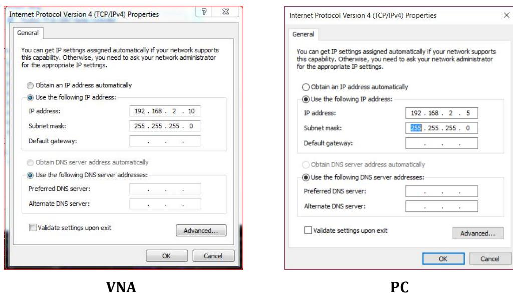
FIGURE 6. SETTING VNA AND PC NETWORK
