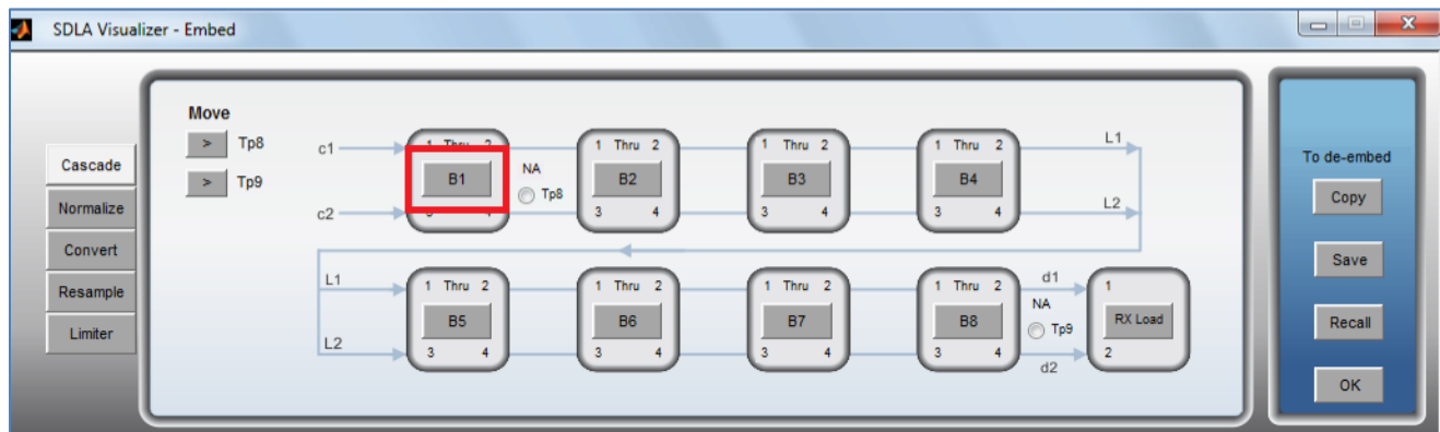
FIGURE 73. CREATE SMA CABLE DE-EMBEDDING + TP3 EMBEDDING FILES – #2
