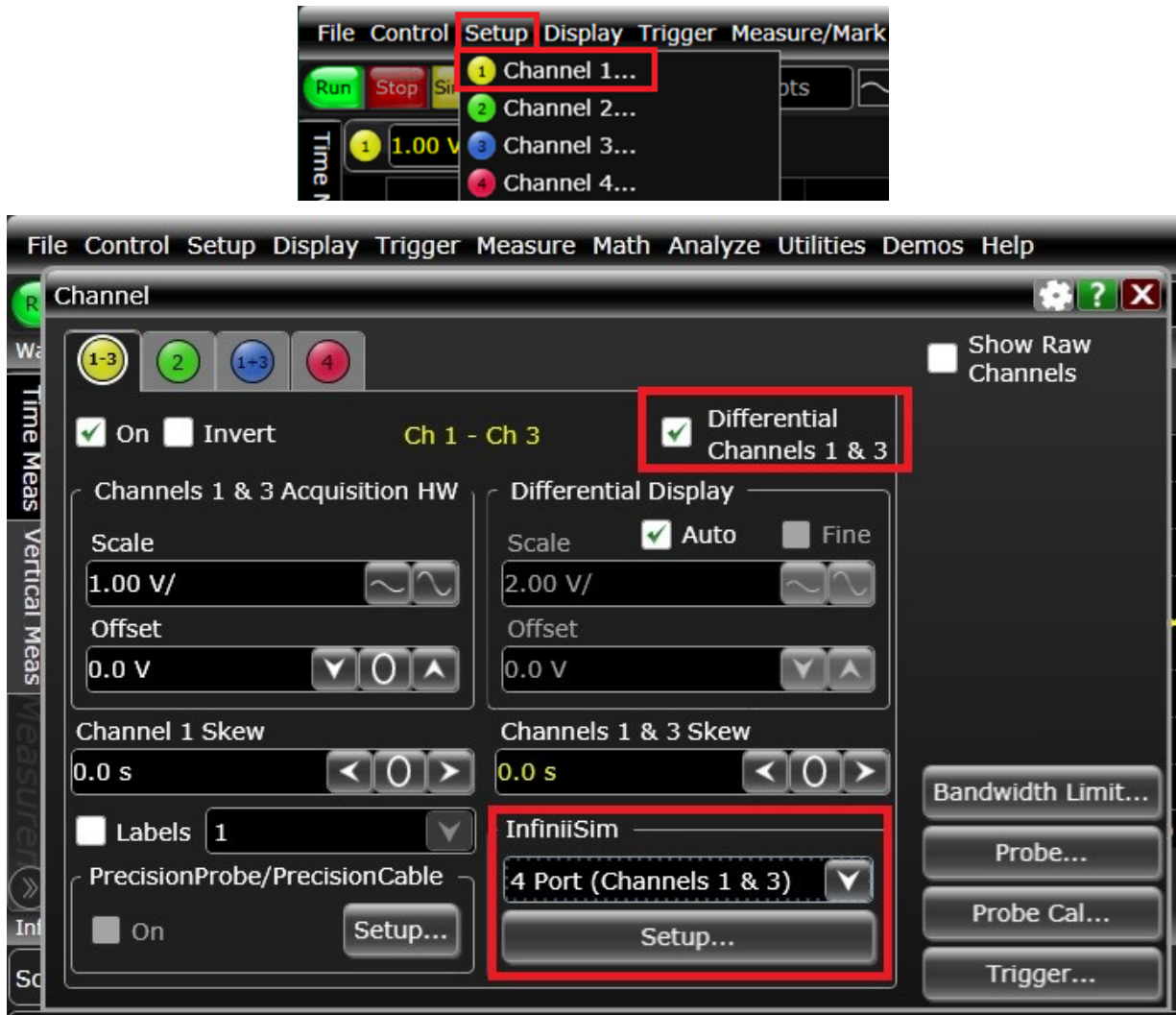
FIGURE 52. SMA CABLE TRANSFER FUNCTION– SET UP SCOPE CHANNELS 1 & 3
