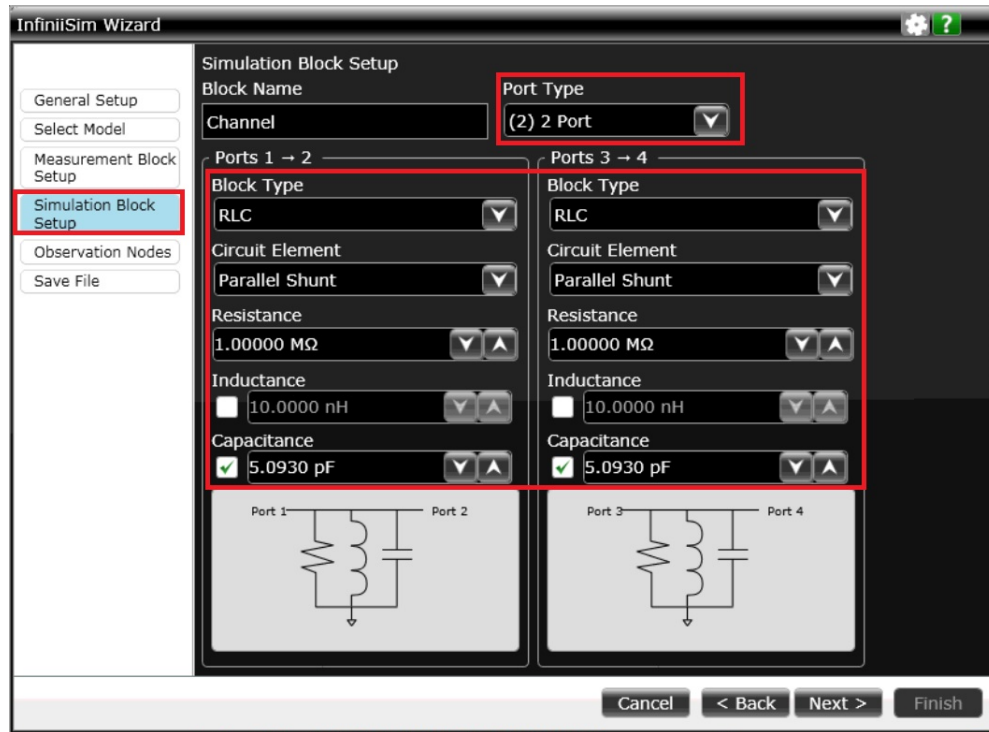
FIGURE 59. SMA CABLE TRANSFER FUNCTION– SET UP INFINIISIM ON SCOPE #6
