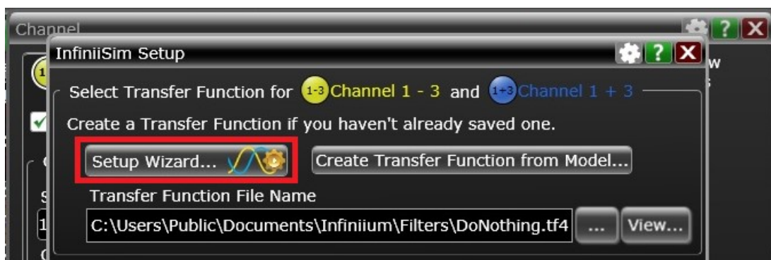
FIGURE 53. SMA CABLE TRANSFER FUNCTION– SELECT SETUP WIZARD ON SCOPE
