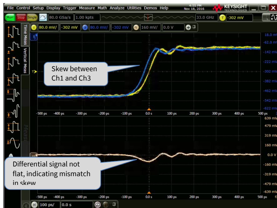
FIGURE 54. SCOPE DE-SKEW OSCILLOSCOPE DISPLAY
