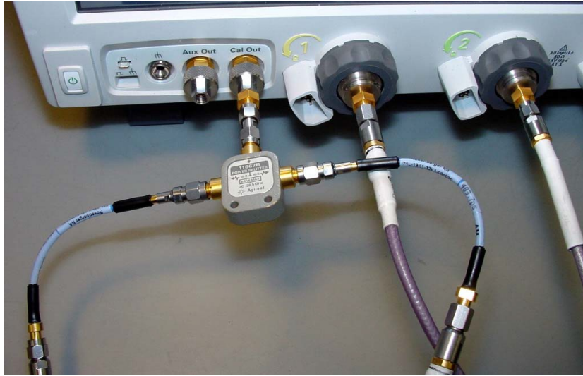
FIGURE 51. SCOPE DESKEW SETUP
