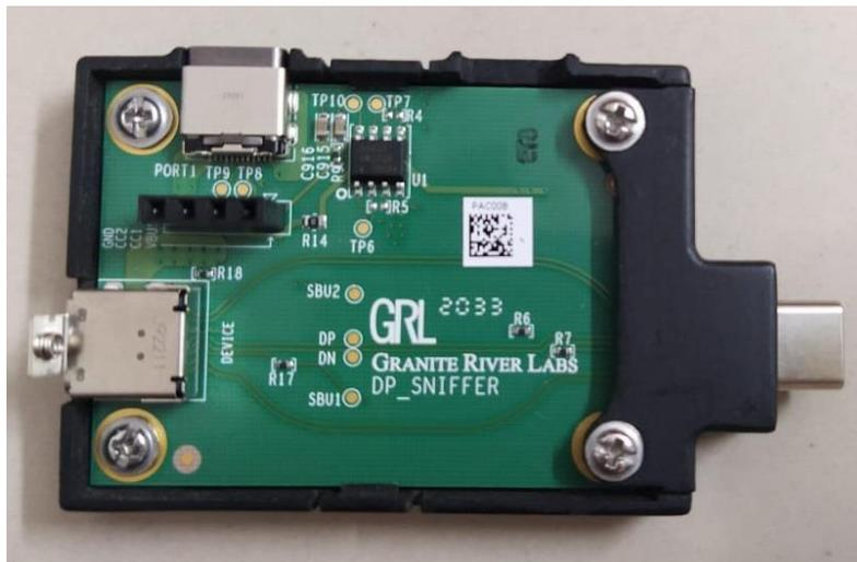
This material is provided as a reference to set up the hardware and software and perform DisplayPort Auxiliary (DP-AUX) transactions using the Granite River Labs DisplayPort Auxiliary Sniffer Board (GRL-C2-DP-AUX-SNIF) and GRL-USB-PD-C2 / C2-EPR test controller as main equipment via the GRL USB Type-C Power Delivery Tester and Analyzer (GRL-USB-PD-C2 / C2-EPR) Browser Application.
