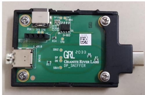
FIGURE 3.6: CLOSE-UP OF GRL-C2-DP-AUX-SNIF BOARD TEST FIXTURE
