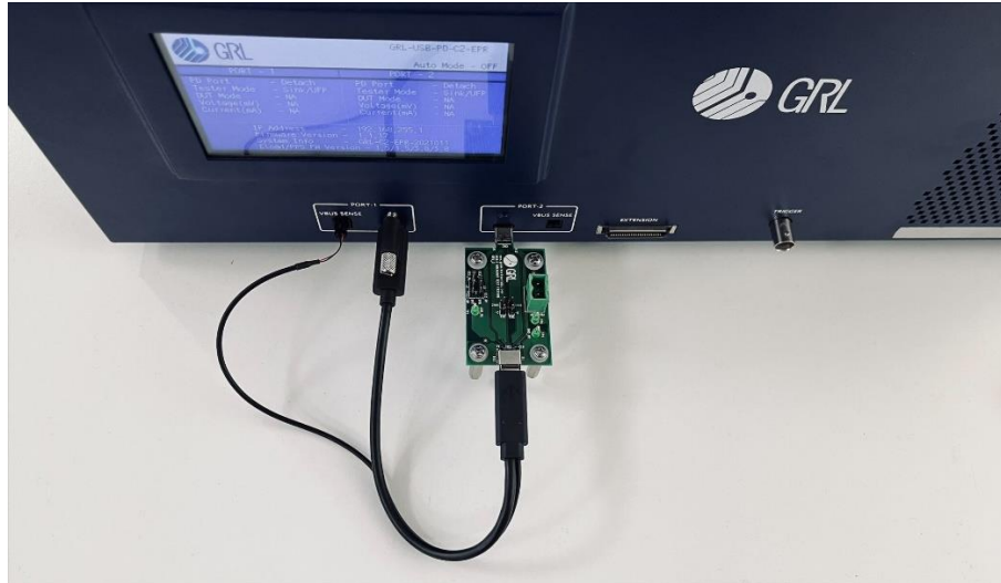
FIGURE 2.1: IEC CONTROLLER SAFETY TEST CONNECTION SETUP
