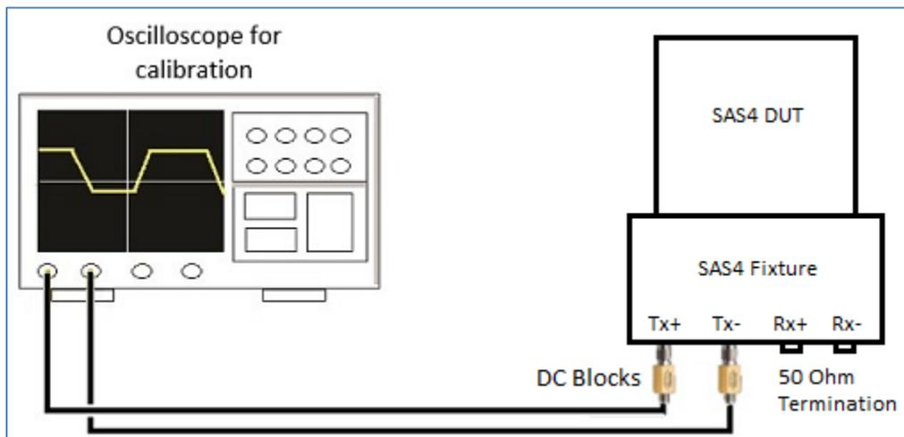
FIGURE 7. COMPLIANCE TEST SETUP FOR TX DUT ZERO-LENGTH TEST LOAD
