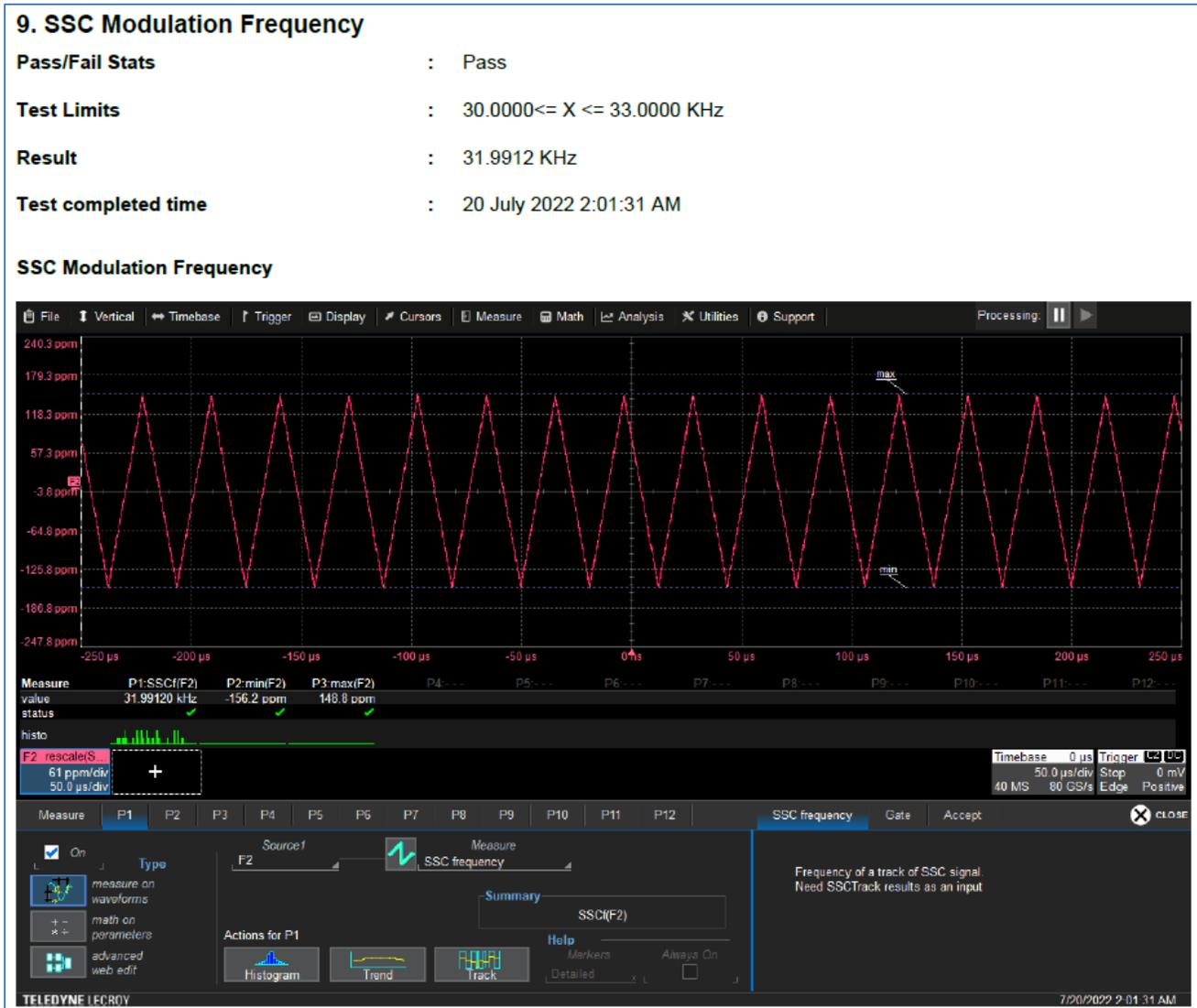
FIGURE 17. TEST RESULTS EXAMPLE
