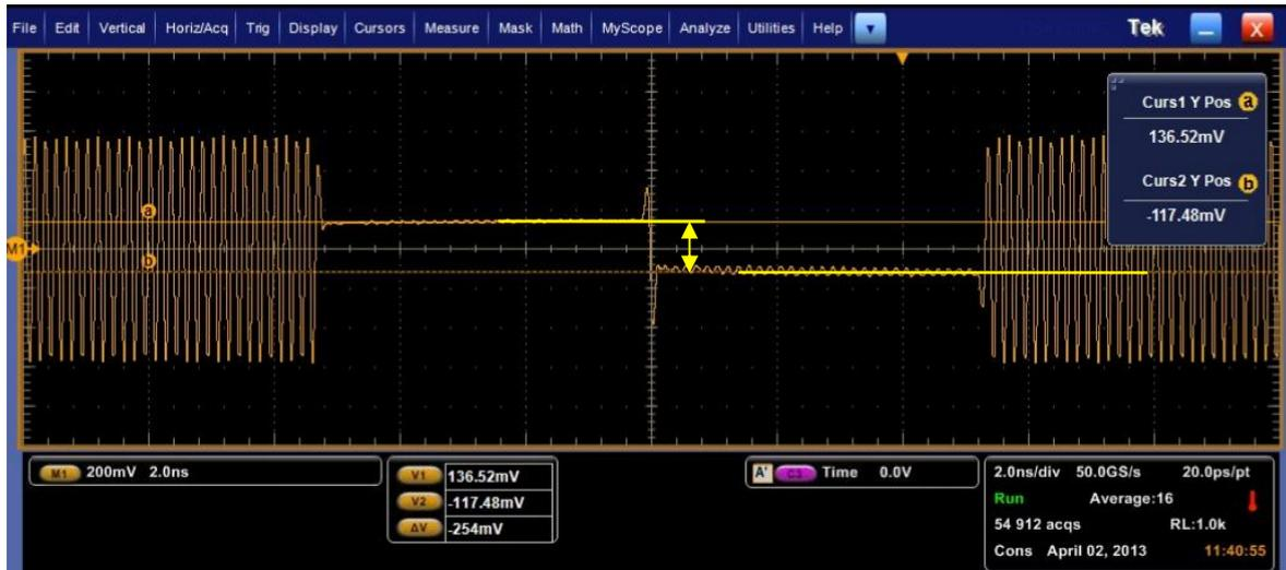
The measured non-transition amplitude in this example is 254mV.
