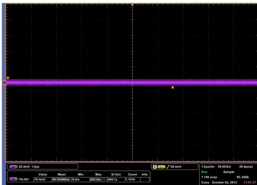
7. Adjust the Clock Amplitude until the amplitude measured is between the maximum 15 to 20mVpp as targeted.
