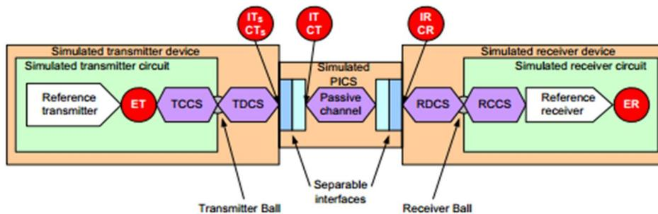
FIGURE 40. SIMULATED 12GBPS TxRx CONNECTION AND COMPLIANCE POINTS
