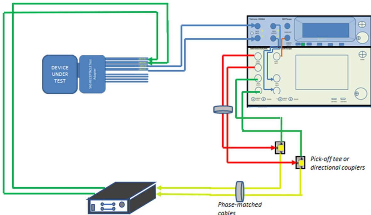
FIGURE 29. COMPLIANCE TEST SETUP FOR RECEIVER DUT JITTER TOLERANCE (USING BSX BERTSCOPE)
