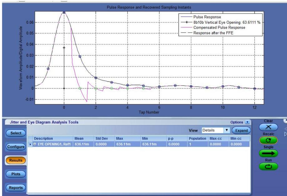
In the above example, the Eye Opening is measured as 63.6% (which is still not within the target range of 65 to 80%). Adjust the ISI Generator accordingly until the expected measurement is obtained.
