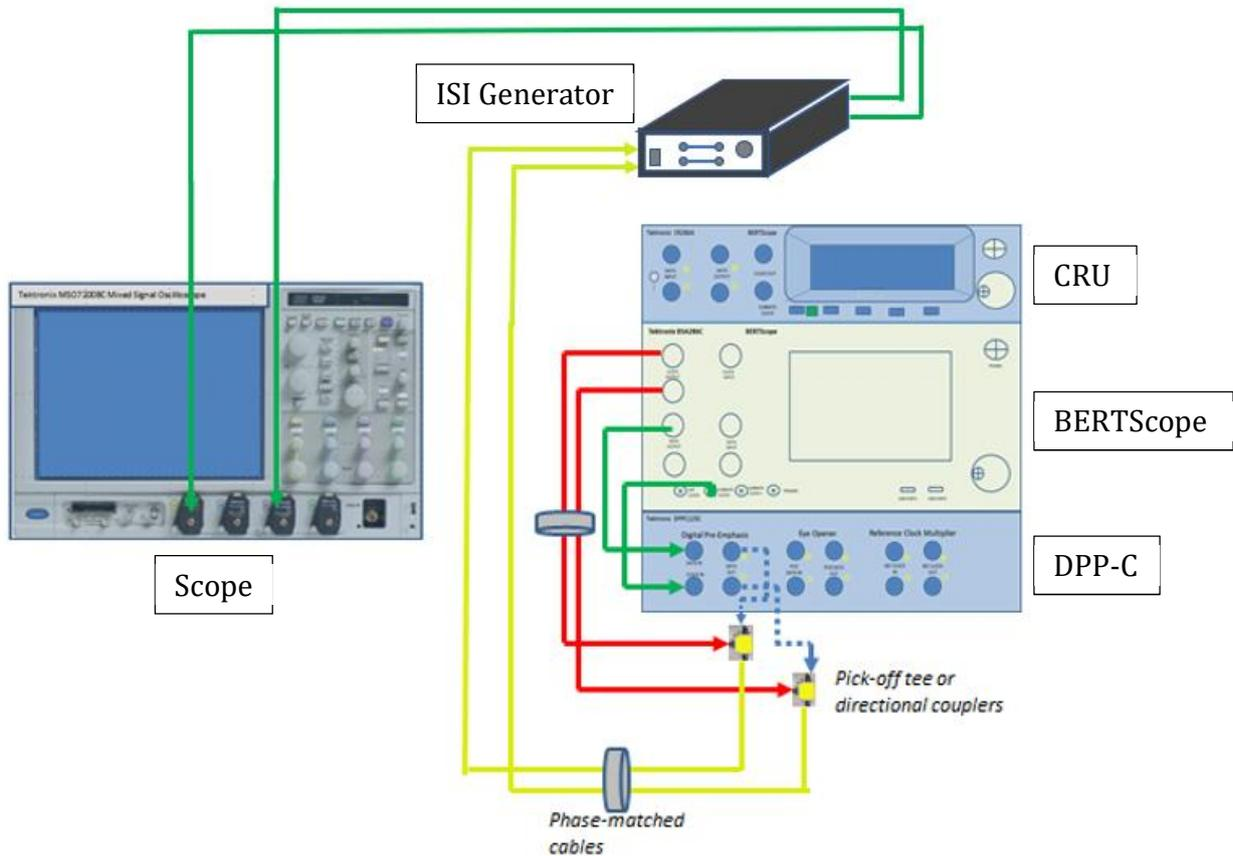
2. Connect the outputs of the ISI Generator to Channel 2 and Channel 4 of the Scope.
