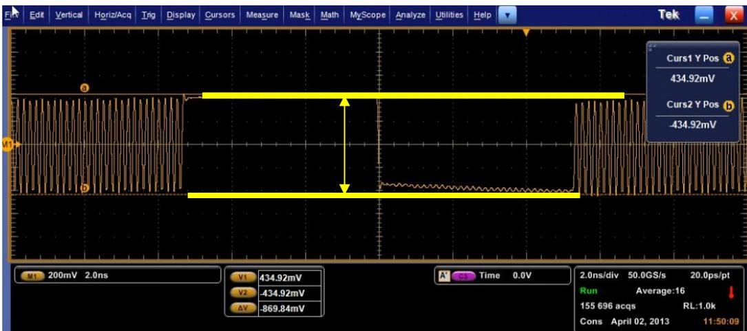
The amplitude measured in this example is 859mVpp, which meets the target.
