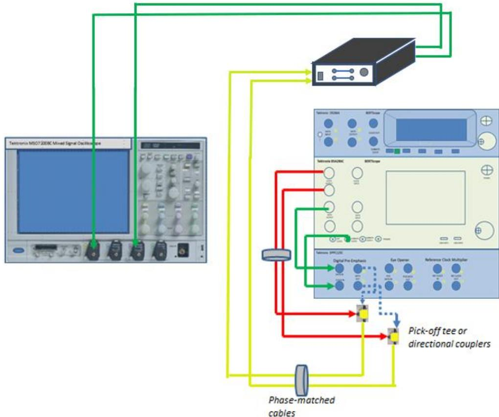
FIGURE 26. EYE OPENING AND CROSSTALK CALIBRATION SETUP (USING BSA BERTSCOPE)
