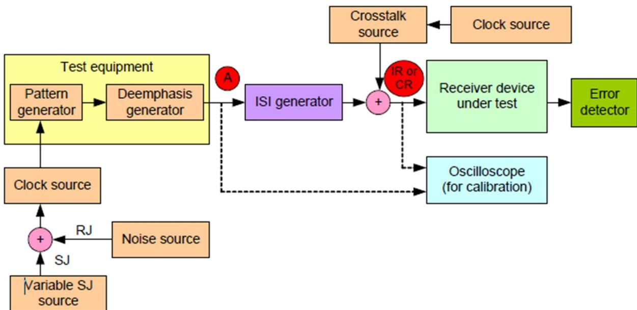
FIGURE 37. TYPICAL STRESSED RX JITTER TOLERANCE TEST/CALIBRATION SETUP BLOCK DIAGRAM
