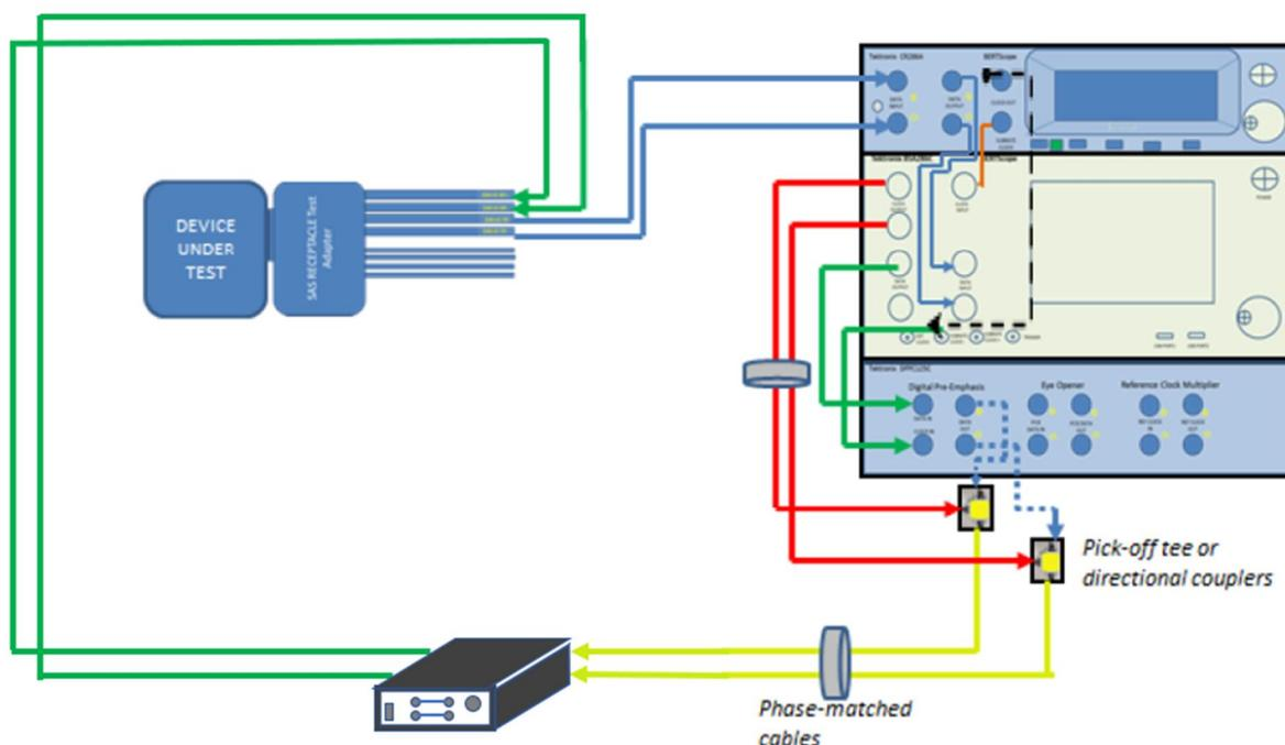
FIGURE 28. COMPLIANCE TEST SETUP FOR RECEIVER DUT JITTER TOLERANCE (USING BSA BERTSCOPE)
