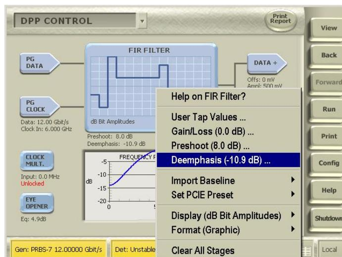
2. Measure the actual de-emphasis and pre-shoot on the scope. Using cursors, measure the peak-to-peak transition amplitude.
