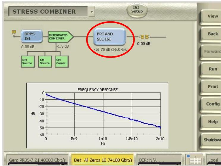
d) Select an initial insertion loss of -12dB. Adjust until the appropriate insertion loss is obtained to approximate the correct Eye Opening as required by the specification.
