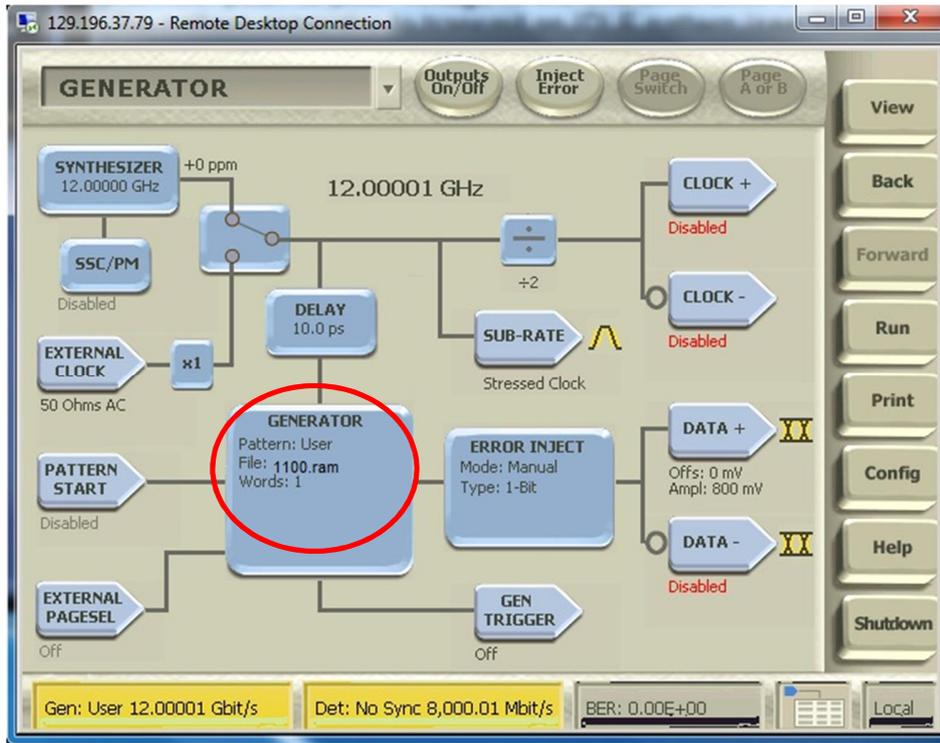
2. Set Random Jitter to 'Intrinsic Limit'. Also enable the Sine Jitter modulator and set the amplitude to 0%UI. The intrinsic jitter generated by the SJ modulator will then be captured in the intrinsic Rj value.
