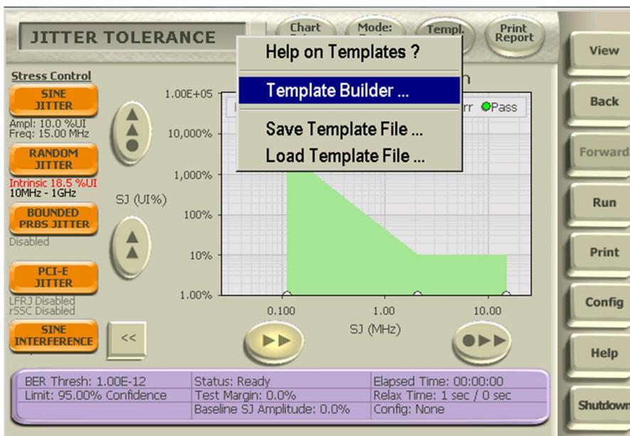
3. Key in the calibrated values for SJ as previously measured.
