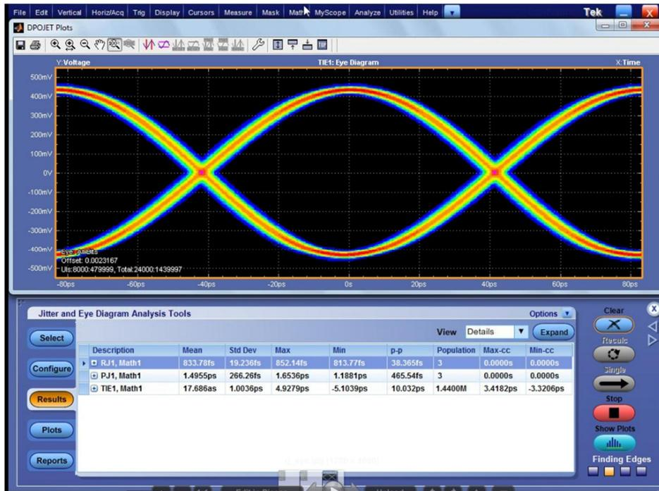
The measured RJ1 value in this example is 0.933ps RMS.
