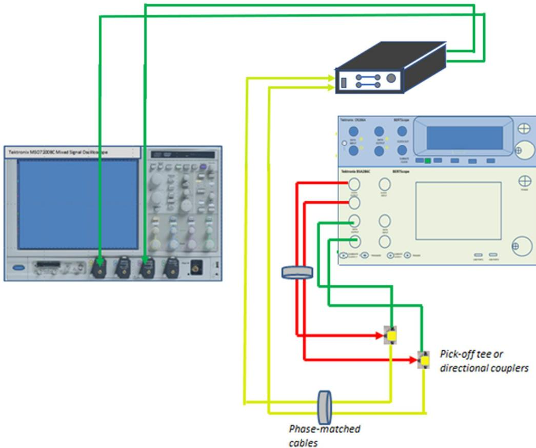
FIGURE 27. EYE OPENING AND CROSSTALK CALIBRATION SETUP (USING BSX BERTSCOPE)
