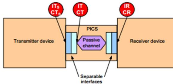
FIGURE 39. 12GBPS TxRx CONNECTION AND COMPLIANCE POINTS
