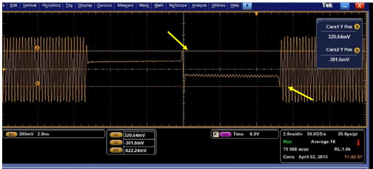
The measured pre-shoot amplitude in this example is 622mV.
