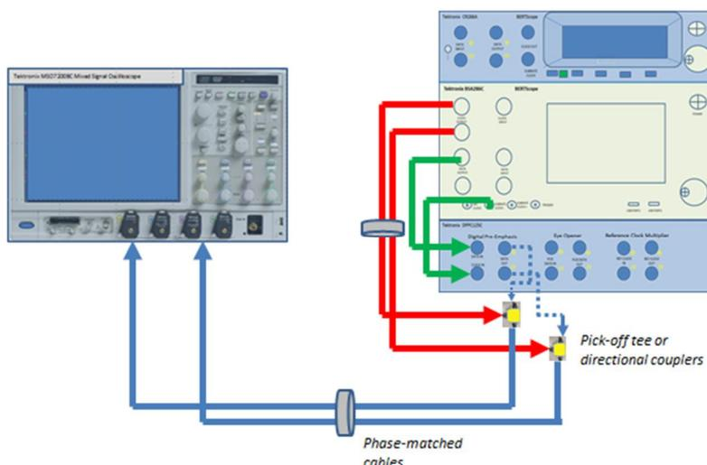
FIGURE 24. SIGNAL AMPLITUDE AND JITTER CALIBRATION SETUP (USING BSA BERTSCOPE)
