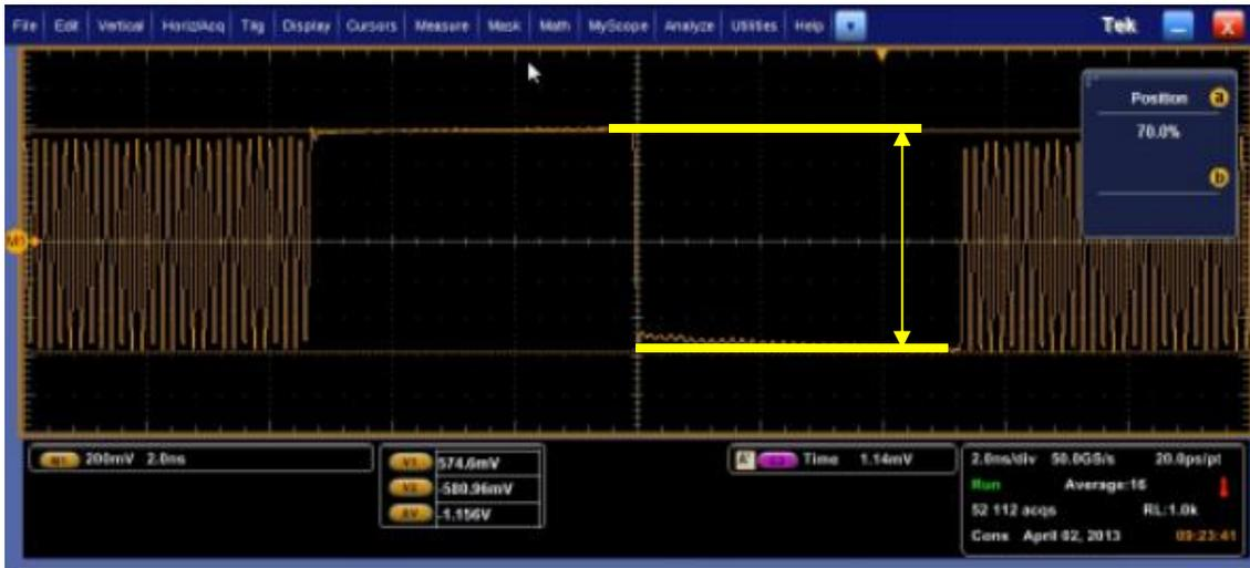
2. Measure the mean AC peak-to-peak amplitude using cursors as 1.134V.
