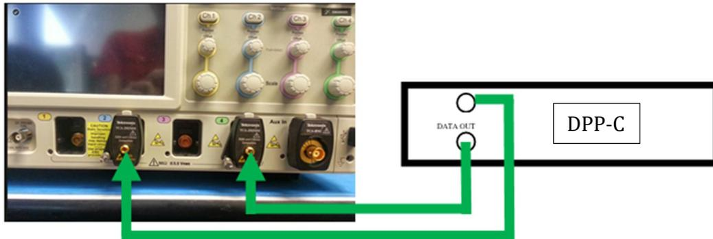
*Note: To generate 25GHz bandwidth, use either Channel 1 and Channel 3 or Channel 2 and Channel 4.*
