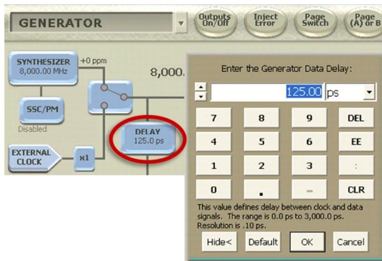
FIGURE 50. GENERATOR DELAY SETTING
