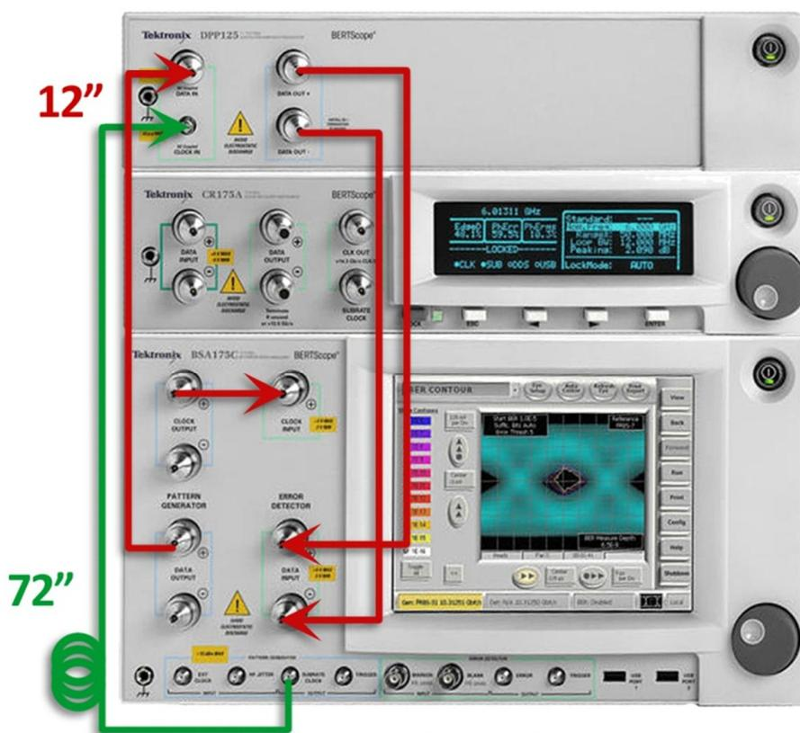
FIGURE 48. CONNECTIONS FOR DPP TIMING CALIBRATION
