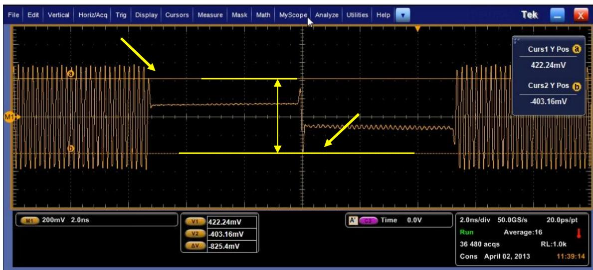
The measured transition amplitude in this example is 825mVpp.
