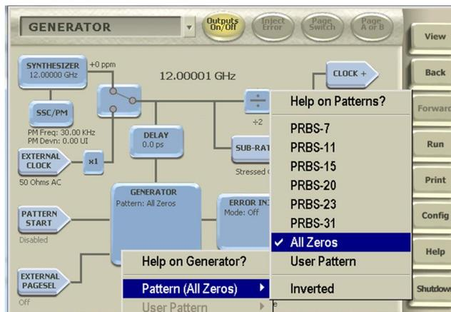
2. On the same page, enable and verify that the BERTScope Clock Output is set to divide-by-2. (Note: While this is automatically performed at 12Gbps, verification is recommended.) The 6GHz Clock supplies a 1010 pattern at 12Gbps.
