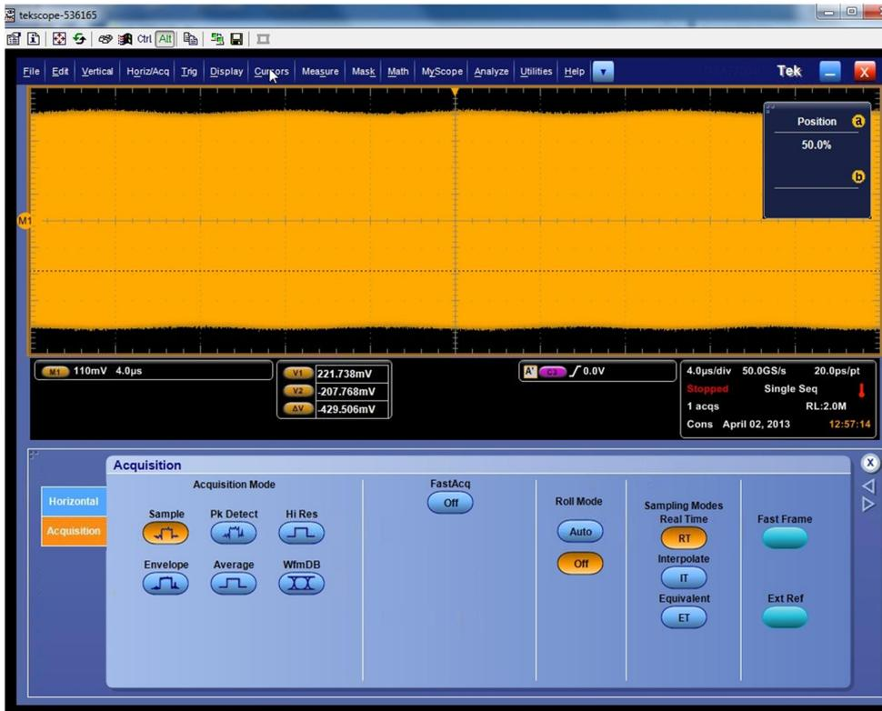
4. Set the Sample Rate to '50GS/s' and the Scale to '4μs/div'.
