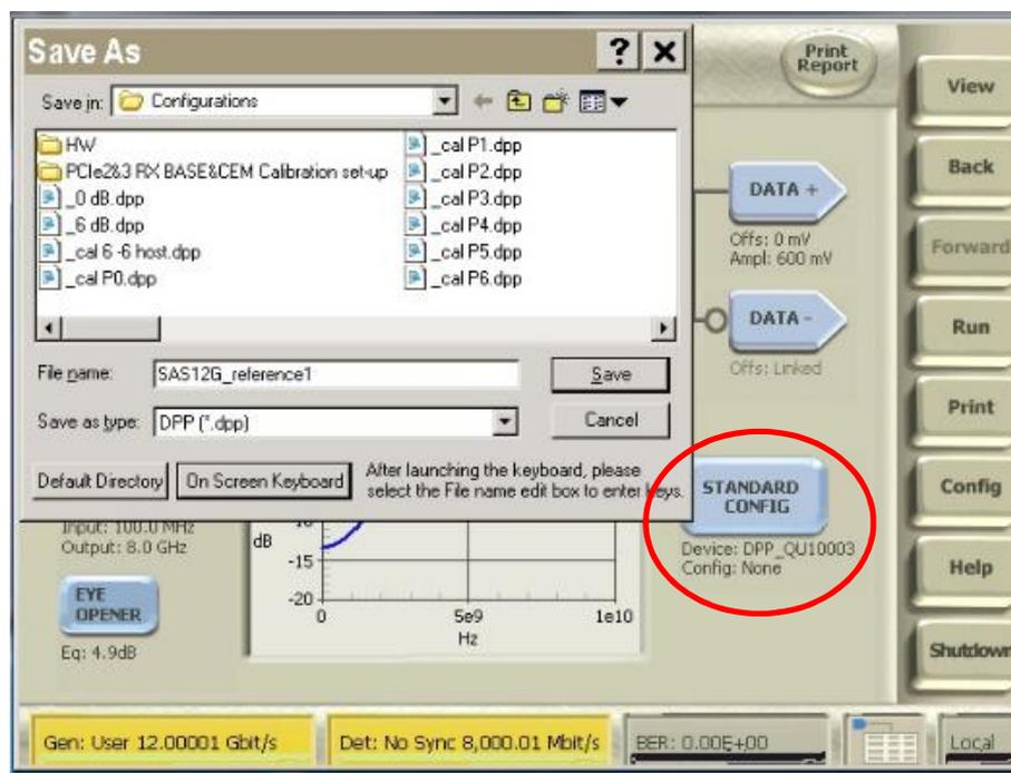
8. Repeat the above calibration and saving procedure for Reference Presets 2 and 3.
