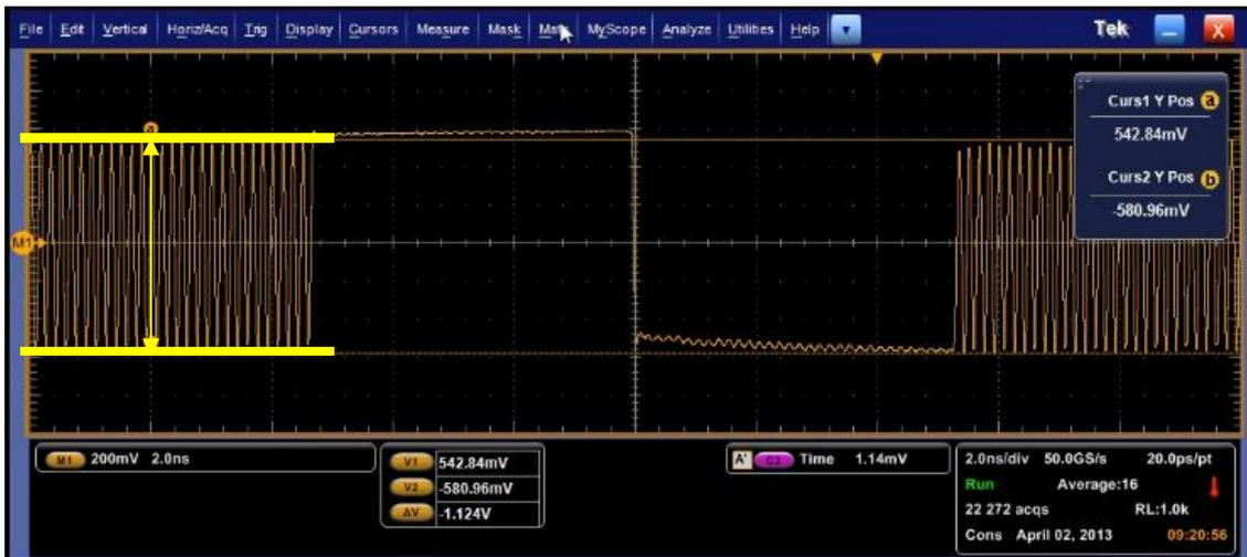
3. Calculate the ratio of HighFrequency/LowFrequency = 1.134V/1.154V = 0.982.
