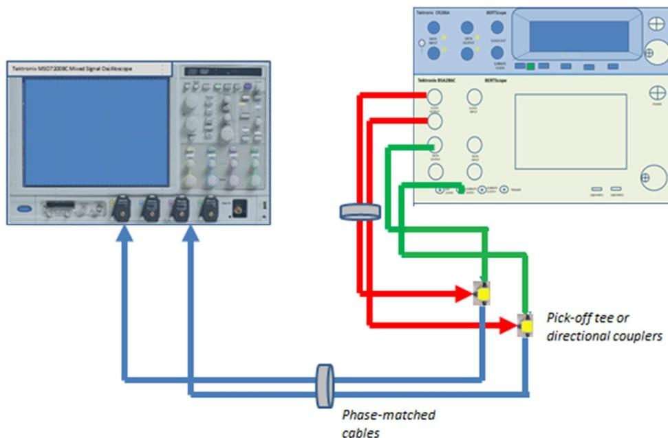
FIGURE 25. SIGNAL AMPLITUDE AND JITTER CALIBRATION SETUP (USING BSX BERTSCOPE)
