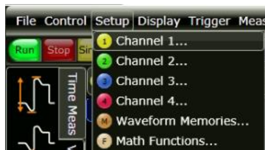
FIGURE 64. SCOPE DE-SKEW PROCESS – OPEN CHANNEL WINDOW
