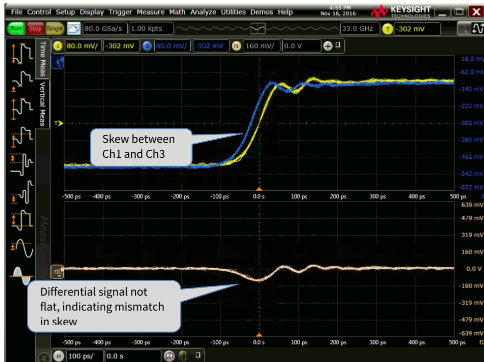
FIGURE 62. SCOPE DE-SKEW OSCILLOSCOPE DISPLAY
