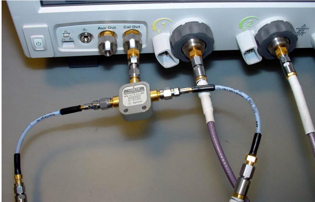
FIGURE 59. SCOPE DESKEW SETUP
