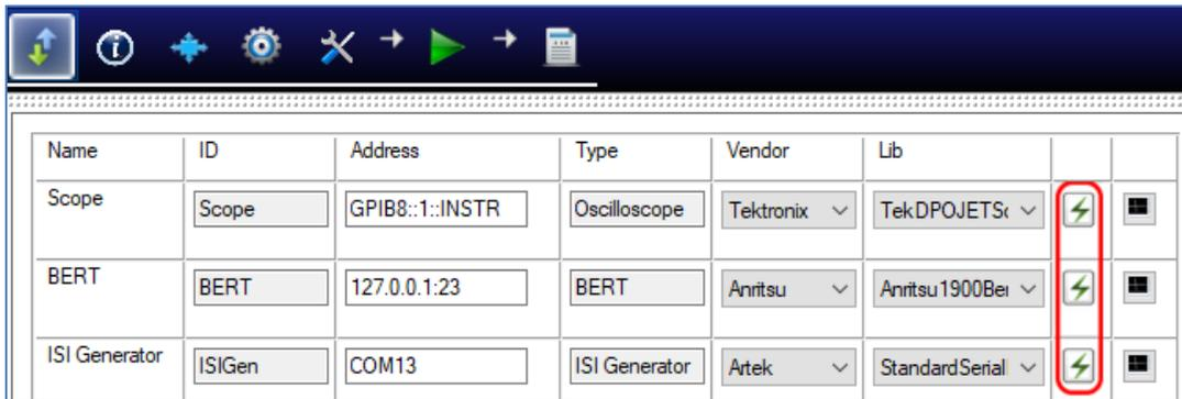
FIGURE 5. CONNECT INSTRUMENTS WITH GRL SOFTWARE
