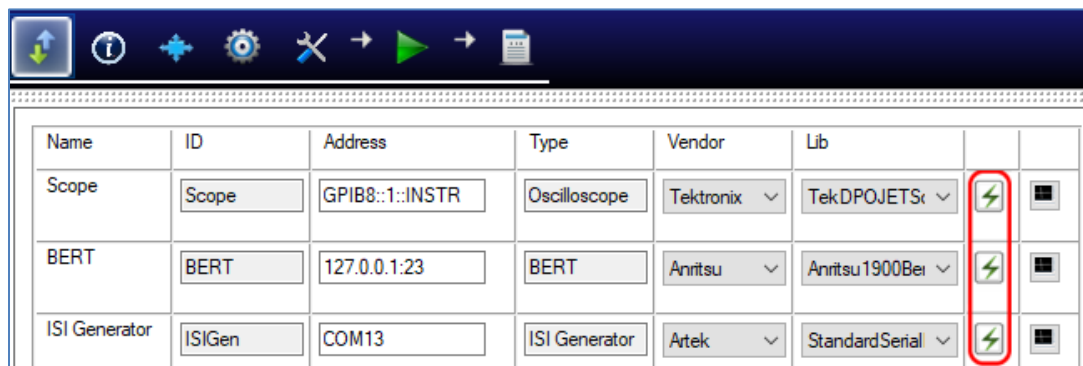
FIGURE 5. CONNECT INSTRUMENTS WITH GRL SOFTWARE
