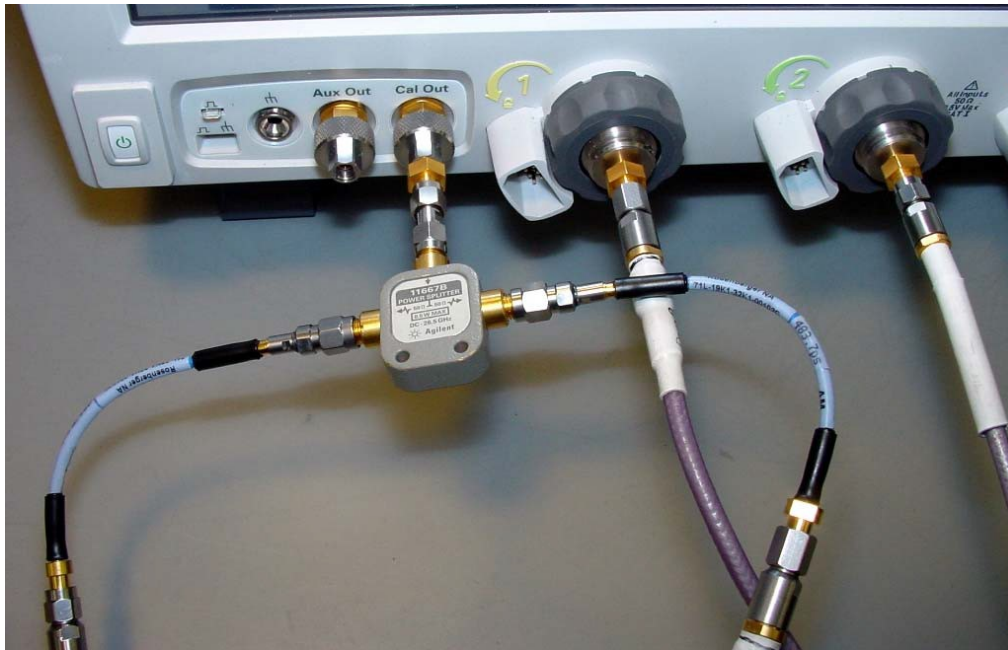
FIGURE 73. SCOPE DESKEW SETUP
