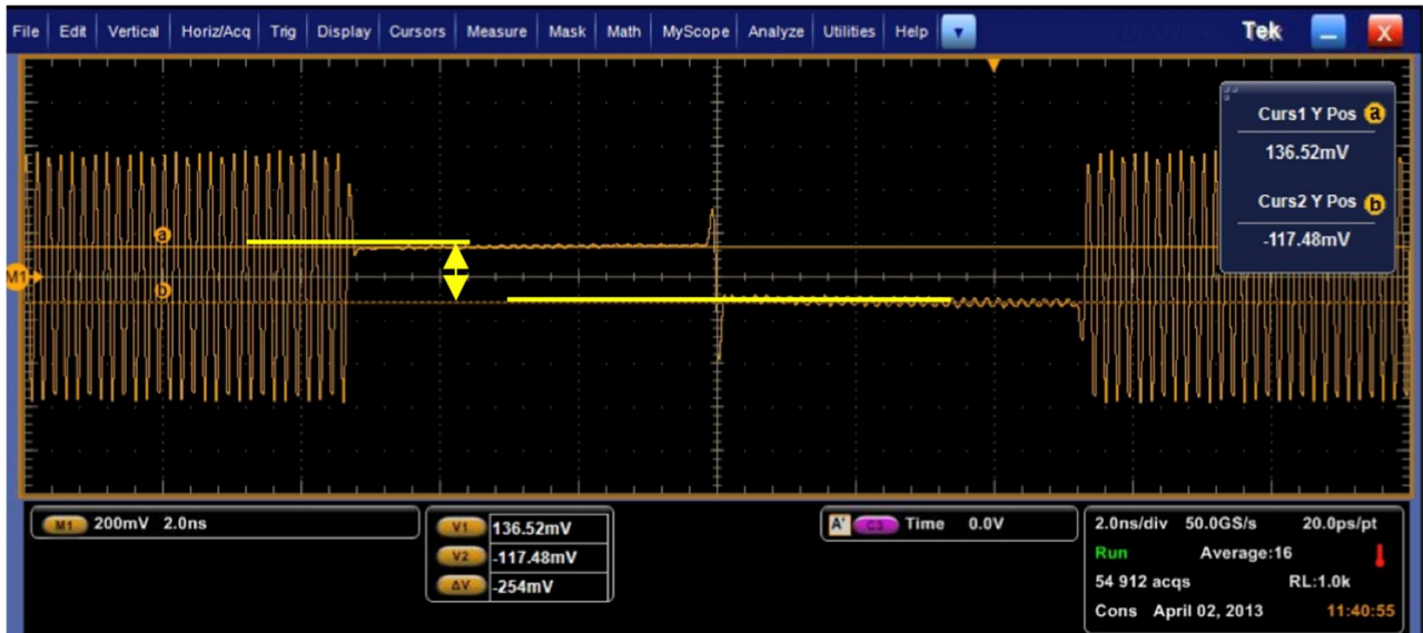
FIGURE 59. MEASURED NON-TRANSITION AMPLITUDE (EXAMPLE 254mV)
