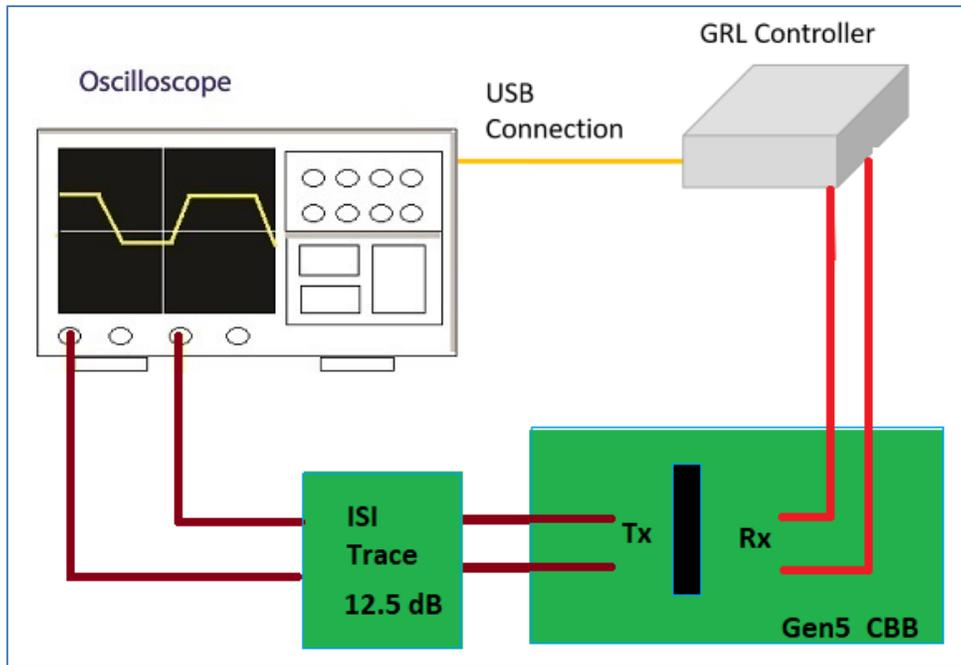
FIGURE 26. CONCEPTUAL PCIe GEN 5 ADD-IN CARD TX TEST SETUP DIAGRAM USING GRL-P1 WITH ISI CHANNEL (WITHOUT RF SWITCH)
