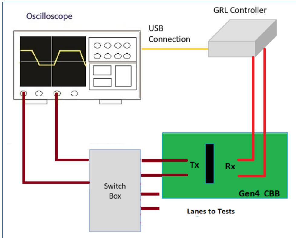
FIGURE 21. CONCEPTUAL PCIe GEN 4 ADD-IN CARD TX TEST SETUP DIAGRAM USING GRL-P1 (WITH RF SWITCH)
