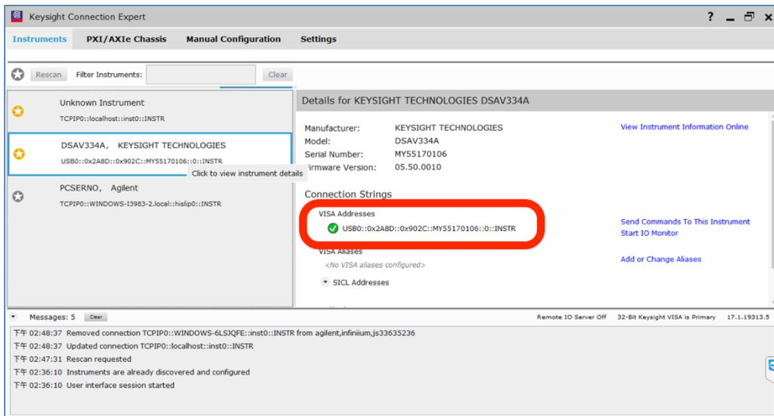
FIGURE 49. OSCILLOSCOPE'S VISA ADDRESS
