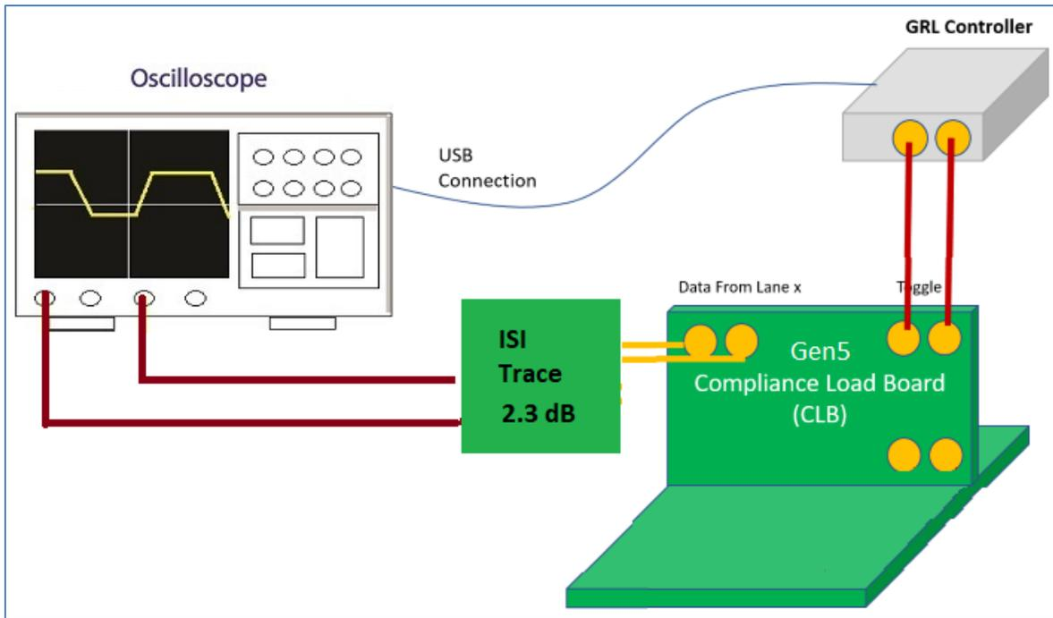
FIGURE 16. CONCEPTUAL PCIe GEN 5 SYSTEM BOARD TX TEST SETUP DIAGRAM USING GRL-P1 WITH ISI CHANNEL (WITHOUT RF SWITCH)
