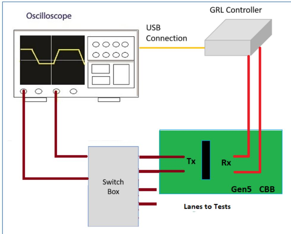
FIGURE 25. CONCEPTUAL PCIe GEN 5 ADD-IN CARD TX TEST SETUP DIAGRAM USING GRL-P1 (WITH RF SWITCH)
