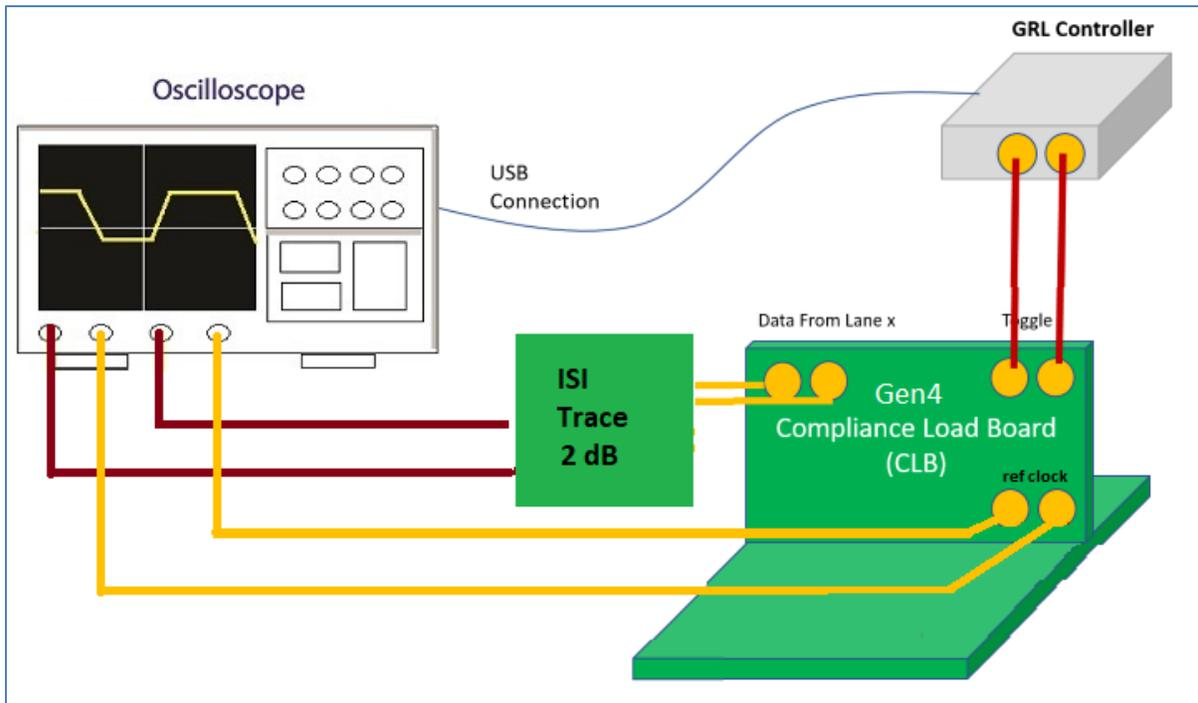
FIGURE 12. CONCEPTUAL PCIe GEN 4 SYSTEM BOARD TX TEST SETUP DIAGRAM USING GRL-P1 WITH ISI CHANNEL (WITHOUT RF SWITCH)
