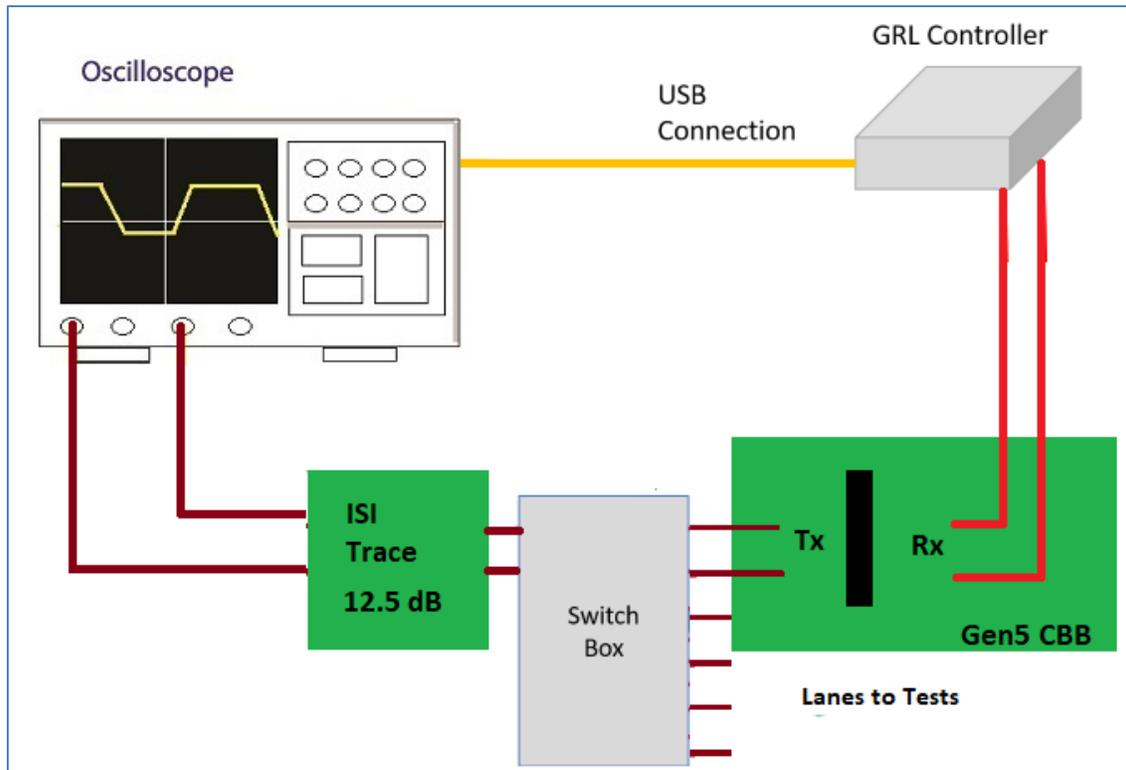
FIGURE 27. CONCEPTUAL PCIe GEN 5 ADD-IN CARD TX TEST SETUP DIAGRAM USING GRL-P1 WITH ISI CHANNEL (WITH RF SWITCH)
