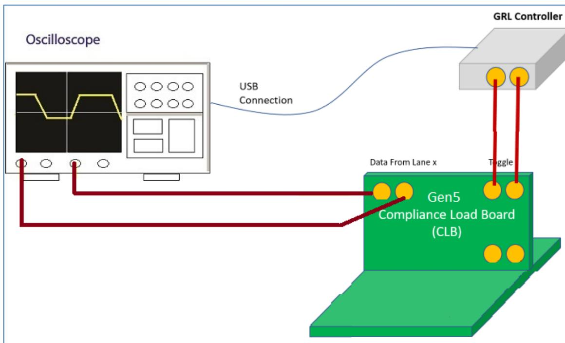
FIGURE 14. CONCEPTUAL PCIe GEN 5 SYSTEM BOARD TX TEST SETUP DIAGRAM USING GRL-P1 (WITHOUT RF SWITCH)
