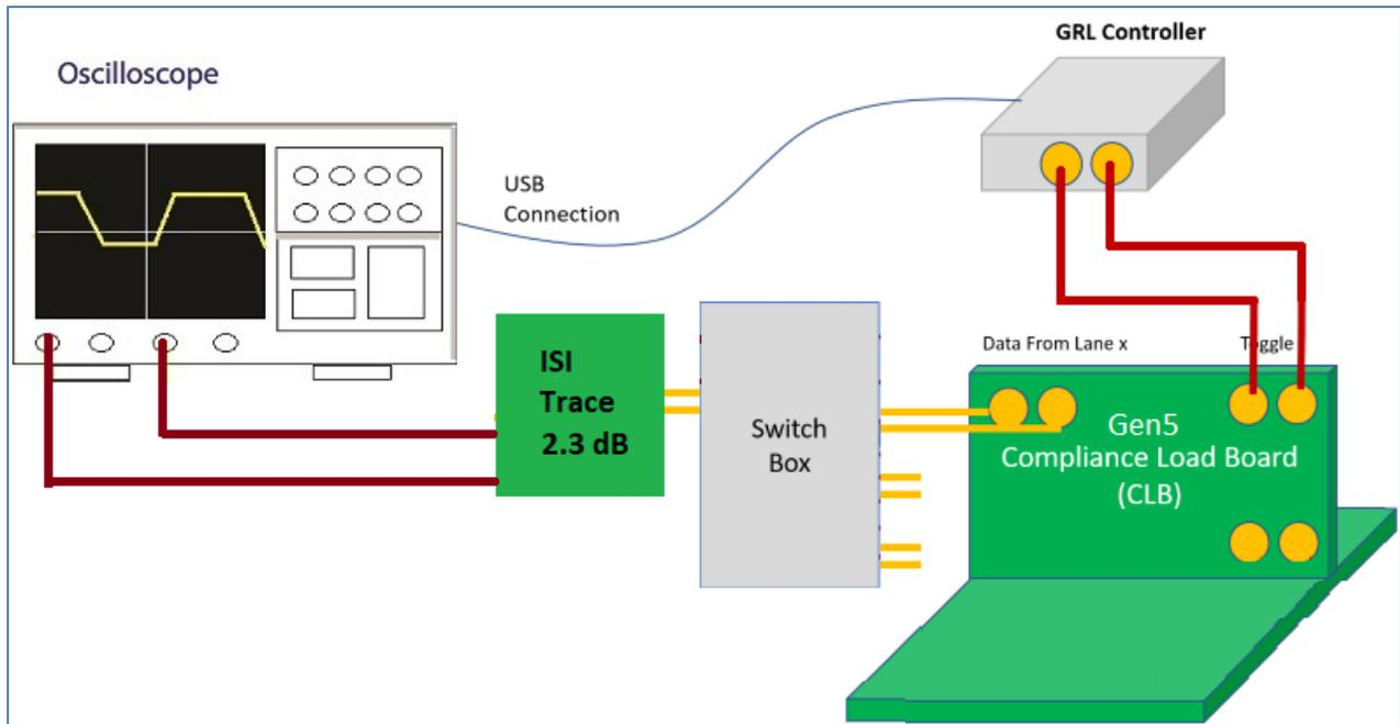
FIGURE 17. CONCEPTUAL PCIe GEN 5 SYSTEM BOARD TX TEST SETUP DIAGRAM USING GRL-P1 WITH ISI CHANNEL (WITH RF SWITCH)
