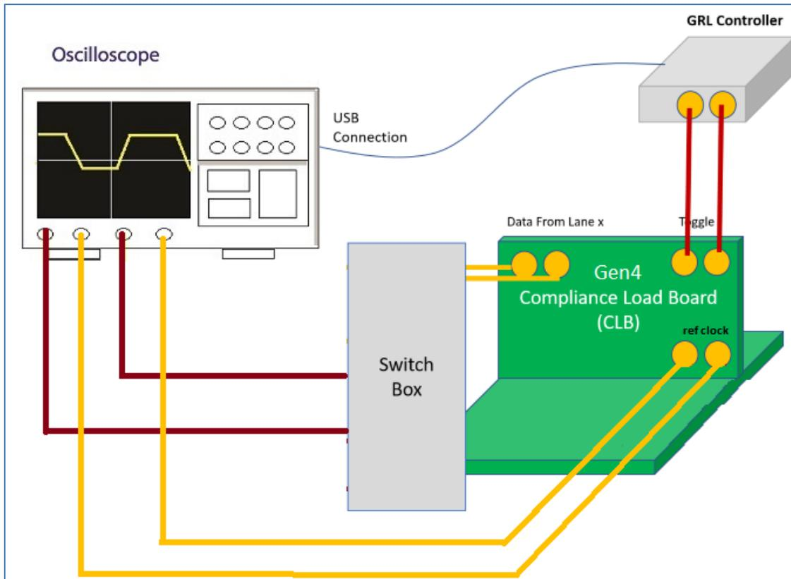
FIGURE 11. CONCEPTUAL PCIe GEN 4 SYSTEM BOARD TX TEST SETUP DIAGRAM USING GRL-P1 (WITH RF SWITCH)
