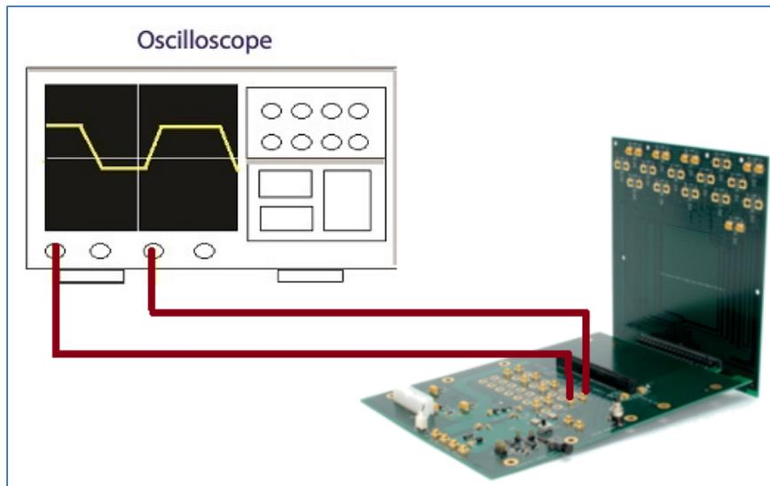
FIGURE 28. CONCEPTUAL PCIe ADD-IN CARD TX TEST SETUP DIAGRAM USING MANUAL COMPLIANCE TOGGLE (WITHOUT RF SWITCH)
