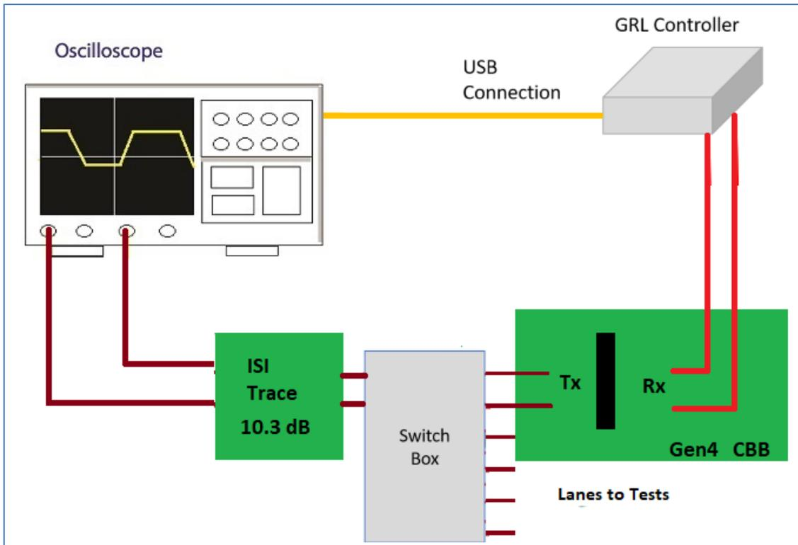
FIGURE 23. CONCEPTUAL PCIe GEN 4 ADD-IN CARD TX TEST SETUP DIAGRAM USING GRL-P1 WITH ISI CHANNEL (WITH RF SWITCH)
