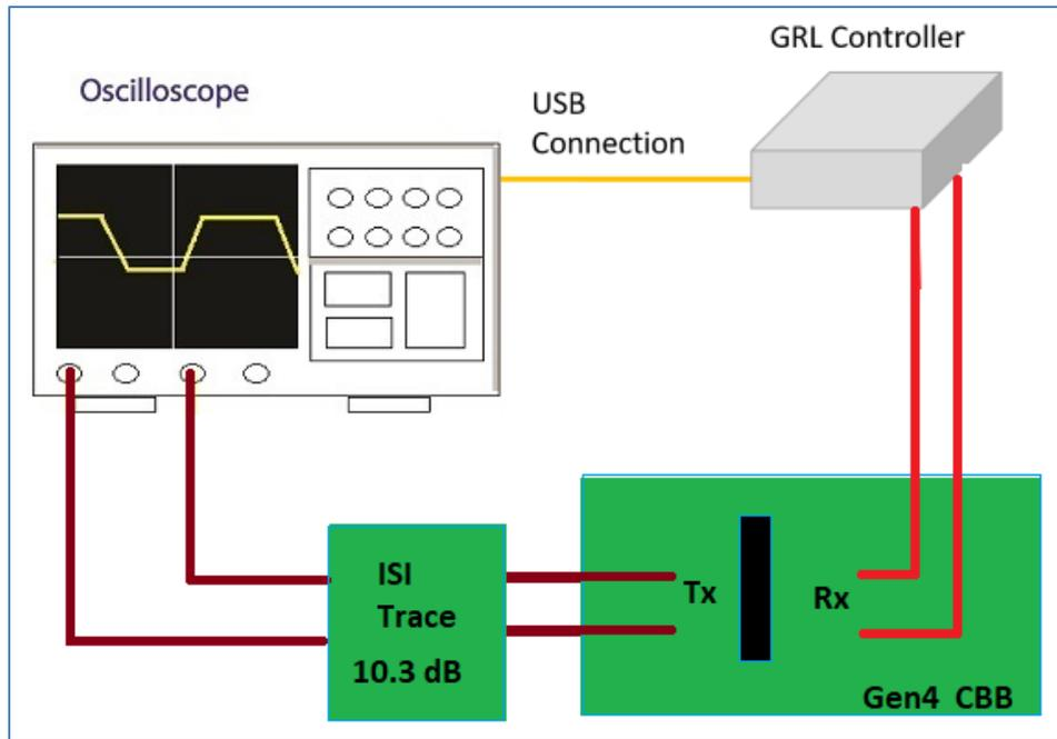
FIGURE 22. CONCEPTUAL PCIe GEN 4 ADD-IN CARD TX TEST SETUP DIAGRAM USING GRL-P1 WITH ISI CHANNEL (WITHOUT RF SWITCH)
