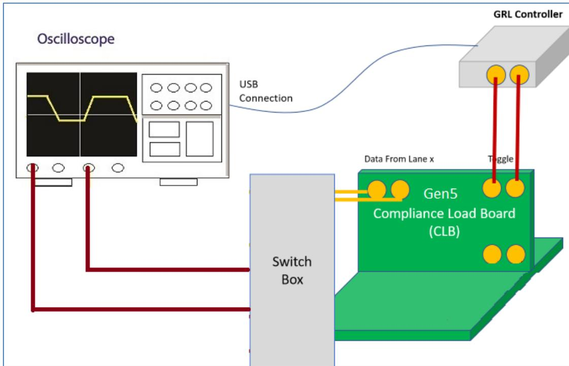
FIGURE 15. CONCEPTUAL PCIe GEN 5 SYSTEM BOARD TX TEST SETUP DIAGRAM USING GRL-P1 (WITH RF SWITCH)
