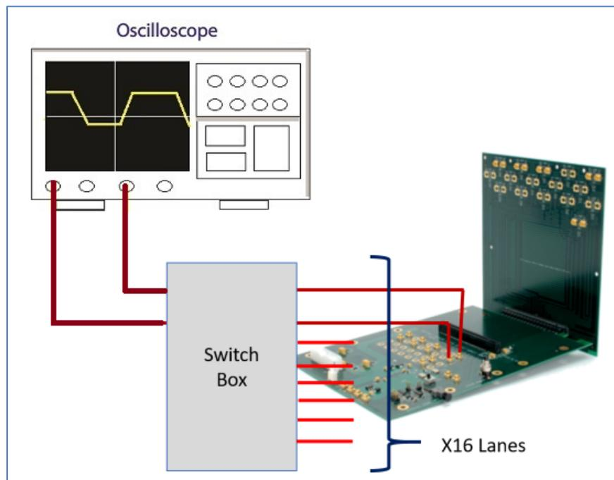
FIGURE 29. CONCEPTUAL PCIe ADD-IN CARD TX TEST SETUP DIAGRAM USING MANUAL COMPLIANCE TOGGLE (WITH RF SWITCH)
