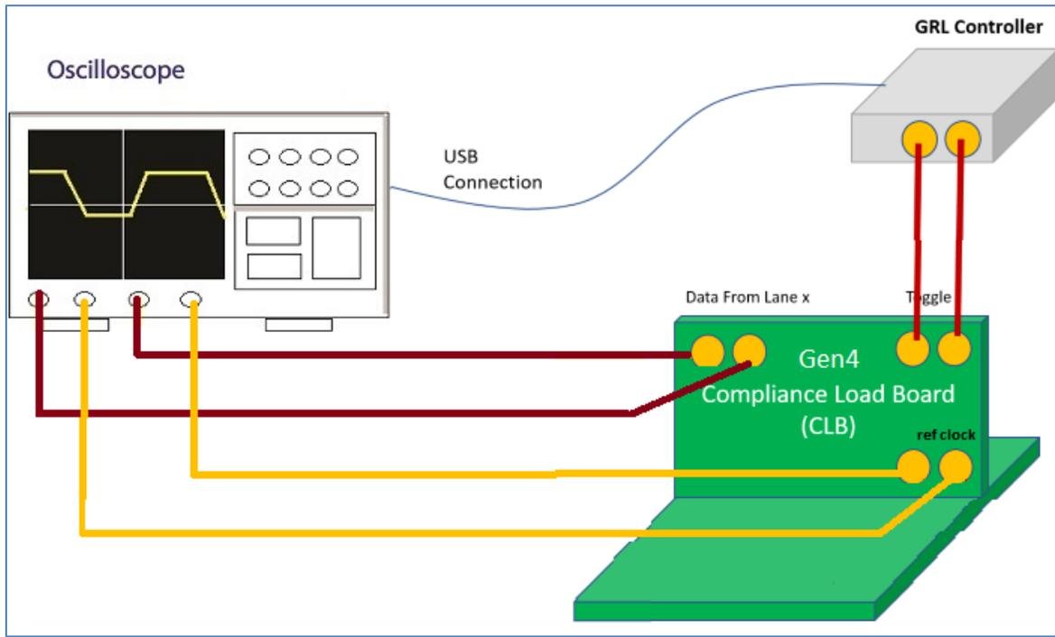
FIGURE 10. CONCEPTUAL PCIe GEN 4 SYSTEM BOARD TX TEST SETUP DIAGRAM USING GRL-P1 (WITHOUT RF SWITCH)
