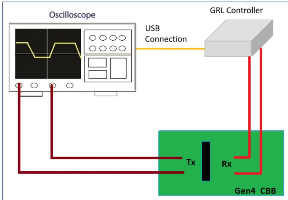
FIGURE 20. CONCEPTUAL PCIe GEN 4 ADD-IN CARD TX TEST SETUP DIAGRAM USING GRL-P1 (WITHOUT RF SWITCH)
