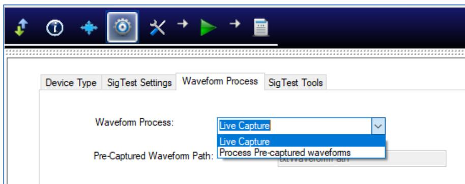
FIGURE 32. SET UP WAVEFORM PROCESSING
