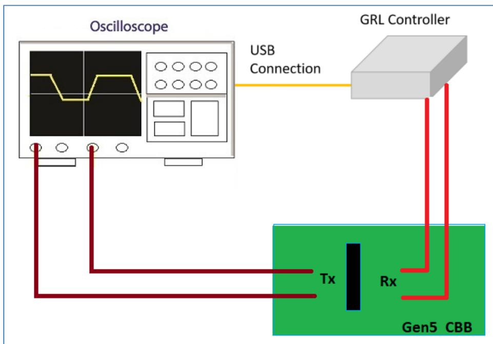
FIGURE 24. CONCEPTUAL PCIe GEN 5 ADD-IN CARD TX TEST SETUP DIAGRAM USING GRL-P1 (WITHOUT RF SWITCH)
