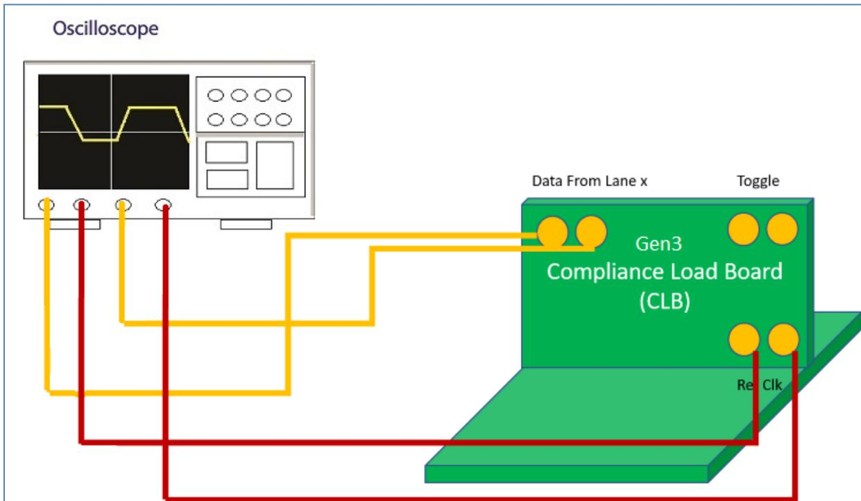
FIGURE 18. CONCEPTUAL PCIe GEN 3 SYSTEM BOARD TX TEST SETUP DIAGRAM USING MANUAL COMPLIANCE TOGGLE (WITHOUT RF SWITCH)
