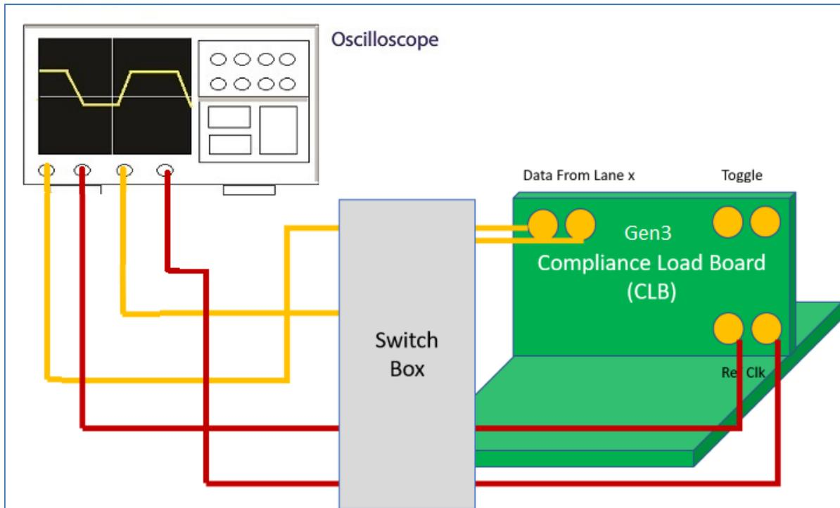
FIGURE 19. CONCEPTUAL PCIe GEN 3 SYSTEM BOARD TX TEST SETUP DIAGRAM USING MANUAL COMPLIANCE TOGGLE (WITH RF SWITCH)
