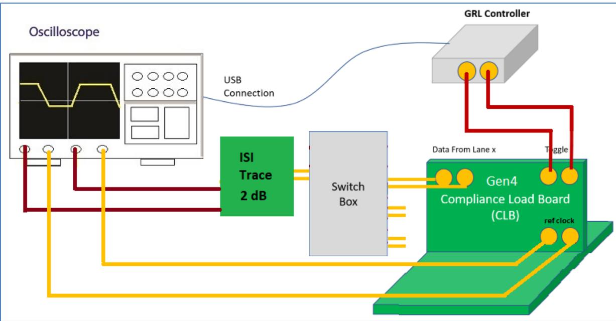
FIGURE 13. CONCEPTUAL PCIe GEN 4 SYSTEM BOARD TX TEST SETUP DIAGRAM USING GRL-P1 WITH ISI CHANNEL (WITH RF SWITCH)
