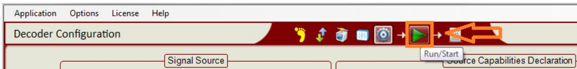
Once you click Run, the decode software takes the inputs from the configuration and decodes the signal. The inbuilt de-serializer creates a stream of data and decodes all the HDMI micro packets.
