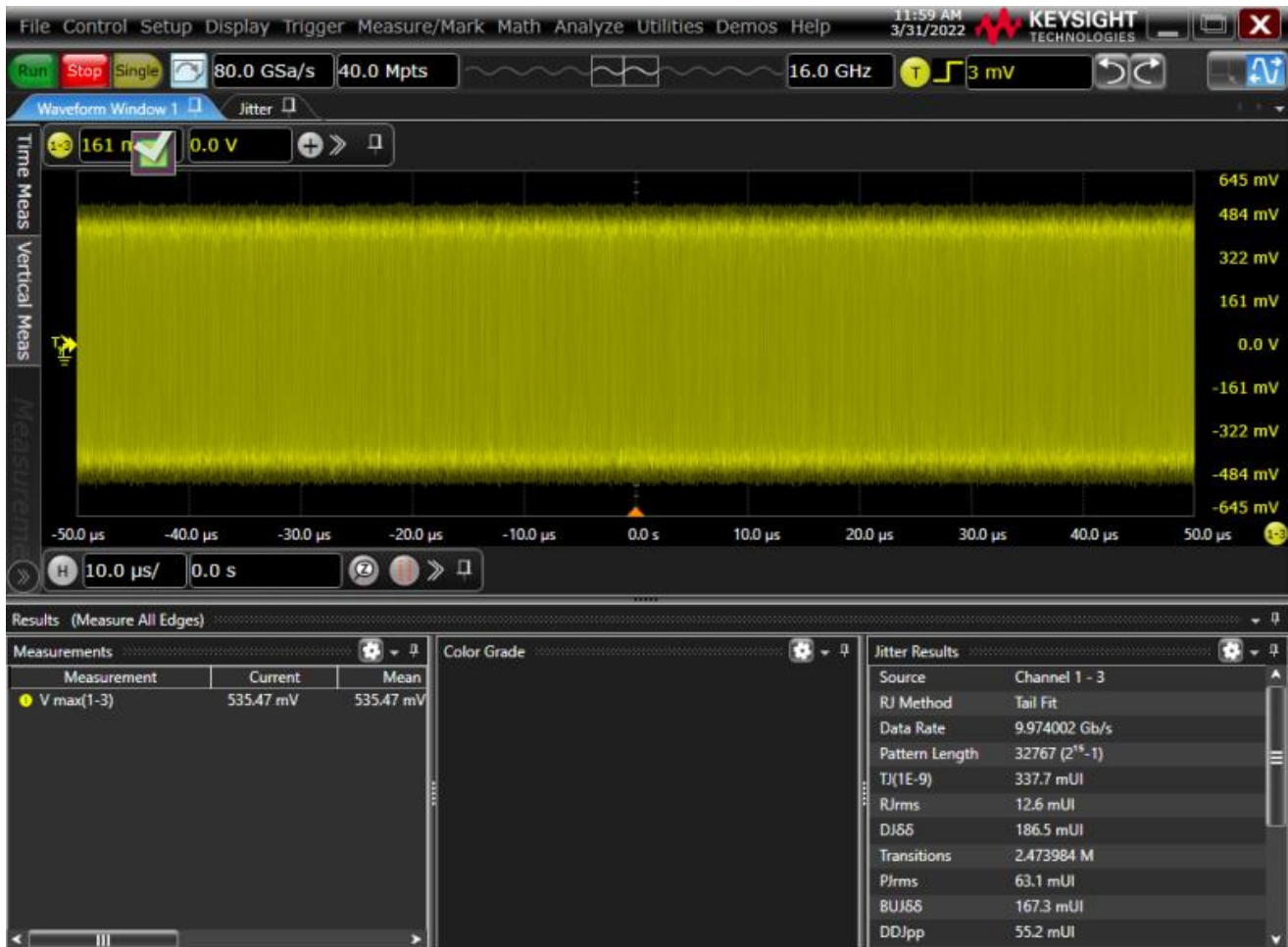
FIGURE 69. TJ MEASUREMENT ON KEYSIGHT SCOPE
