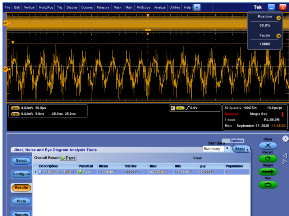
FIGURE 59. CALIBRATION TO PHASE MATCH ON TEKTRONIX SCOPE
