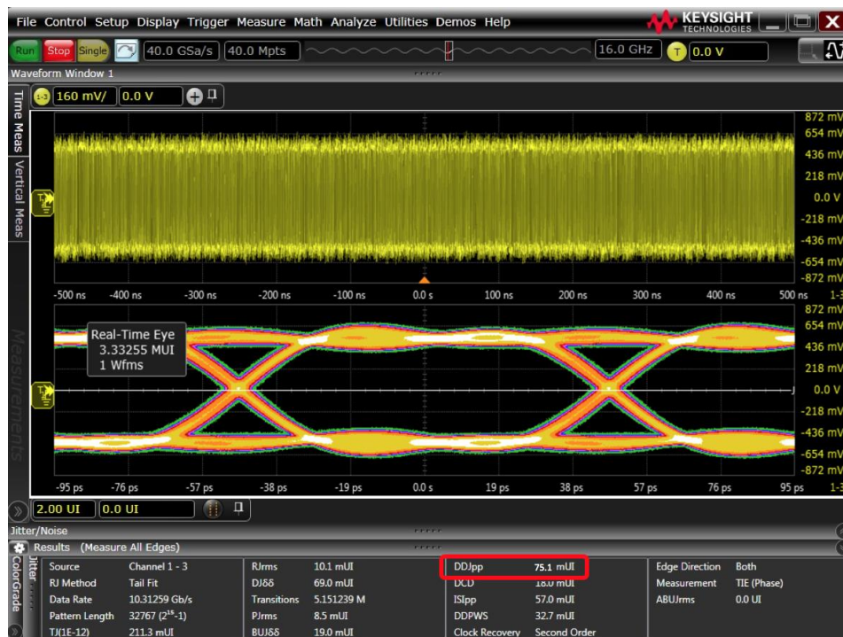
FIGURE 56. OPTIMIZED PRESET (MINIMUM DDJPP) MEASUREMENT ON KEYSIGHT SCOPE
