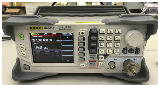
FIGURE 53. DSG815 SJ_{FIXED} ADJUSTMENT EXAMPLE FOR HBR3 AND HBR2
