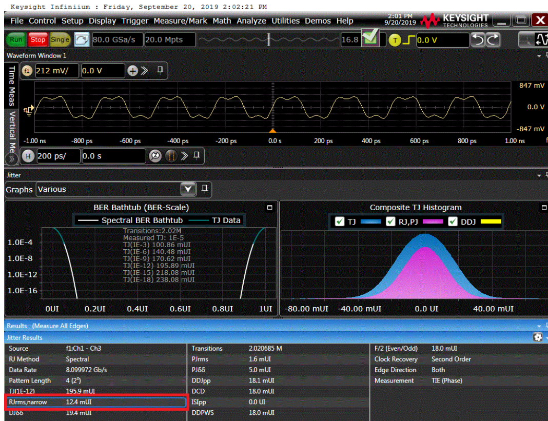
FIGURE 50. HBR3 RJ MEASUREMENT EXAMPLE ON KEYSIGHT SCOPE
