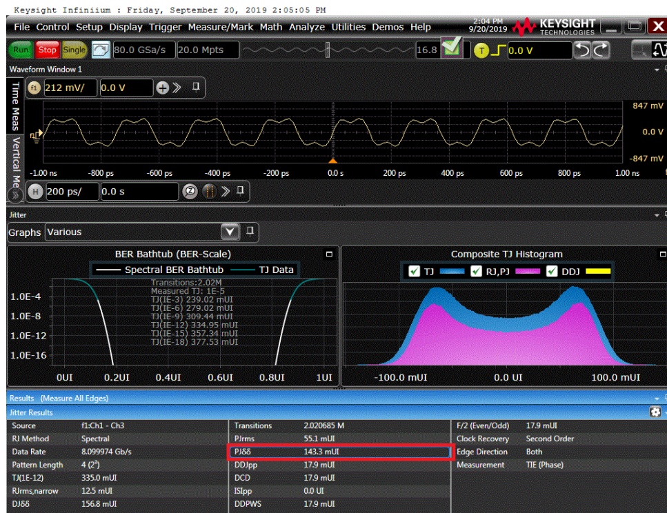
FIGURE 58. HBR3 SJ SWEEP MEASUREMENT EXAMPLE ON KEYSIGHT SCOPE
