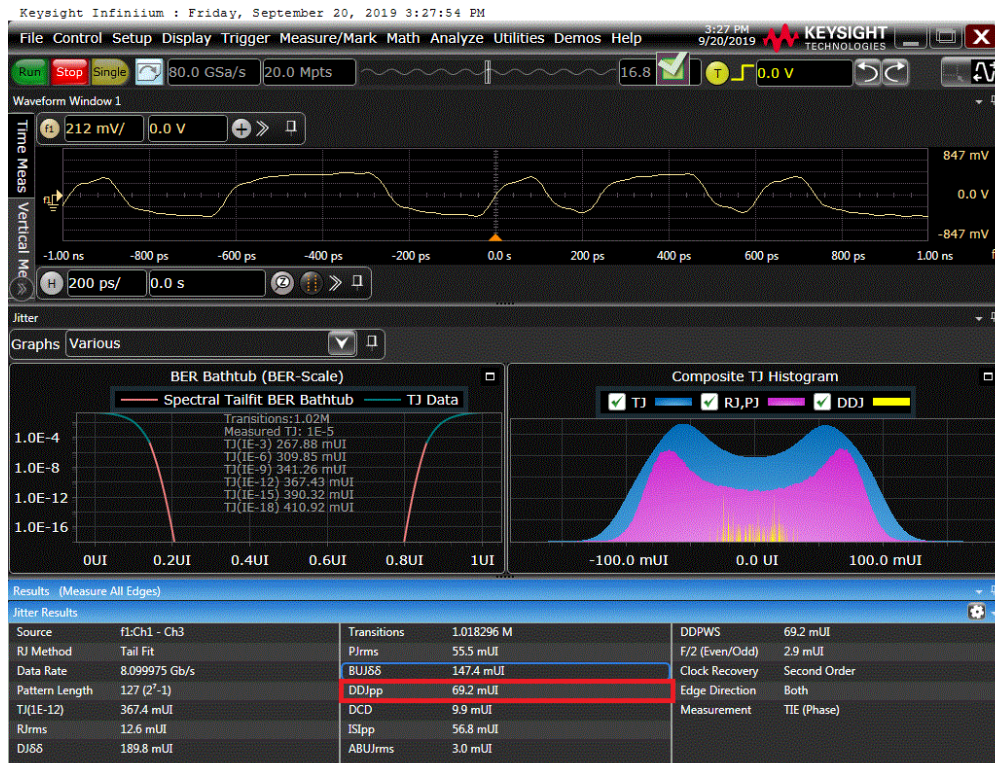
FIGURE 61. HBR3 ISI MEASUREMENT EXAMPLE ON KEYSIGHT SCOPE
