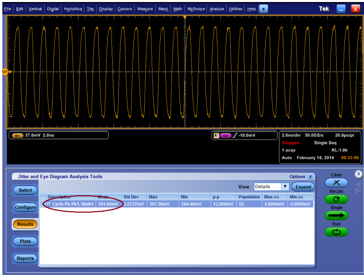
FIGURE 71. HBR2 CROSSTALK MEASUREMENT ON TEKTRONIX SCOPE
