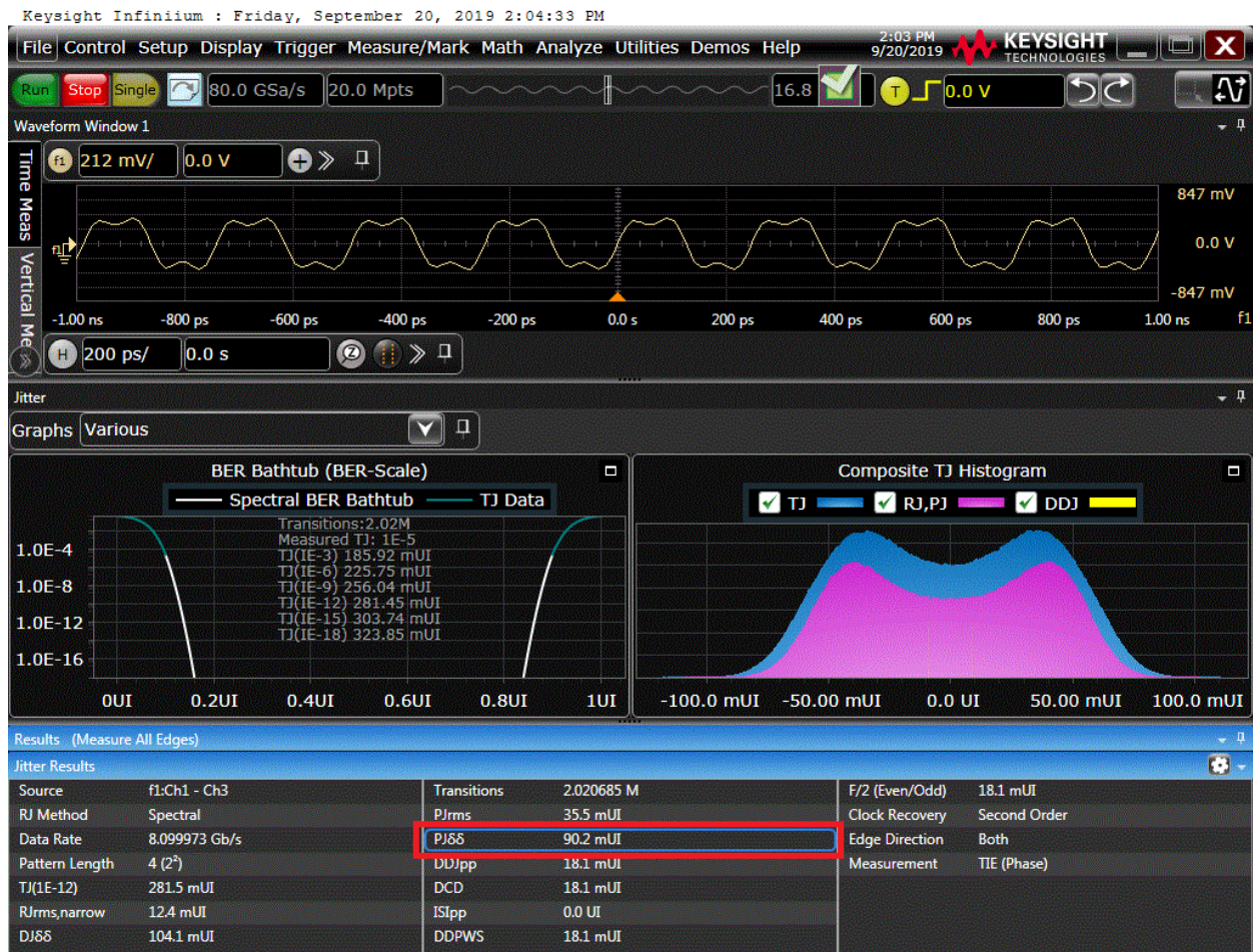
FIGURE 54. HBR3 SJ FIXED MEASUREMENT EXAMPLE ON KEYSIGHT SCOPE (NOT SHOWING TARGET 80mUI)
